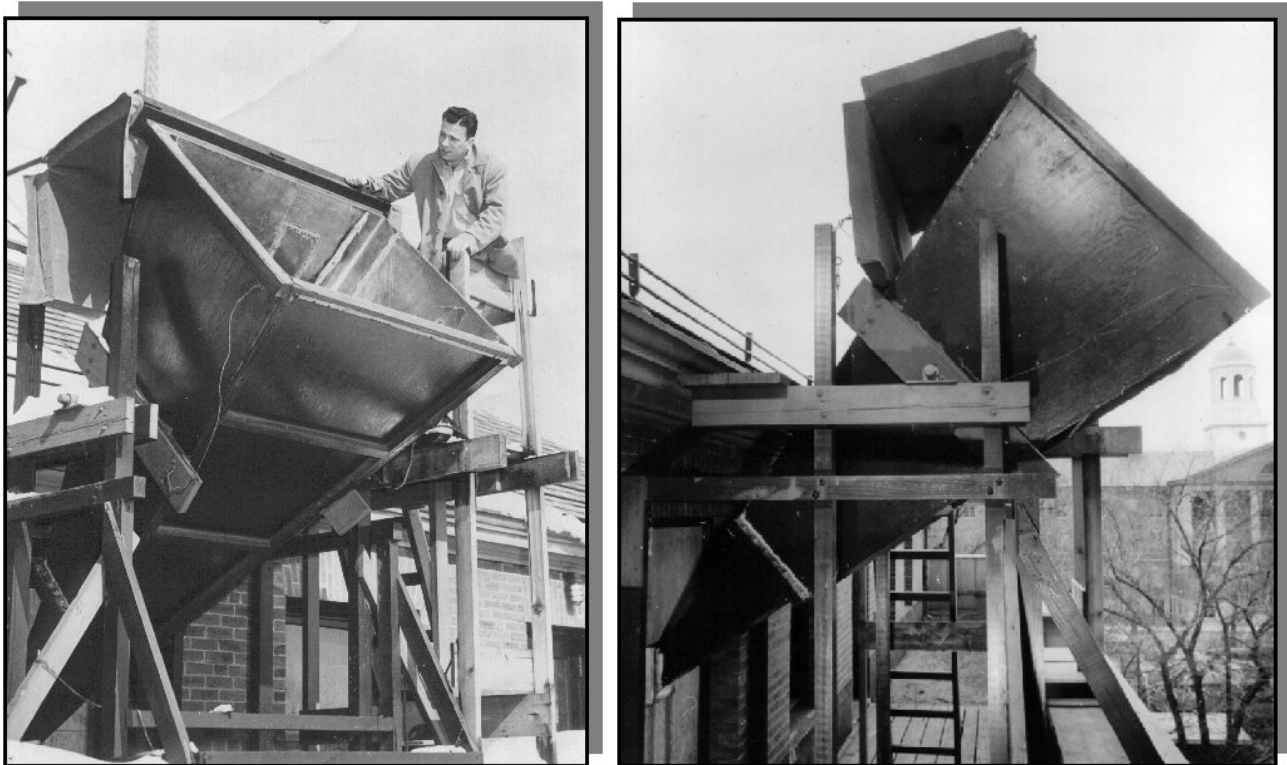
Harold "Doc" Ewen, Ph.D. and Horn Antenna mounted on 4th floor window of Lyman Physics Laboratory at Harvard University Used to Detect Neutral Hydrogen on March 25, 1951
