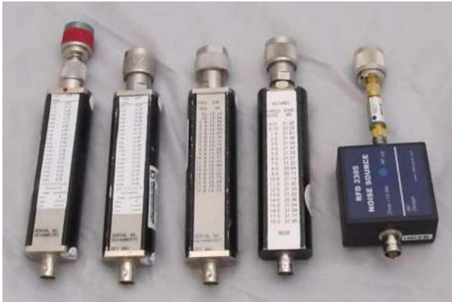
Figure 1 ~ Noise sources, left-to-right in same order as table 1. Note that the RFD2305 (far-right) has a Mini-Circuits 10 dB attenuator on its output. The attenuator adapts the 15 dB ENR of the base unit to 5 dB ENR and also improves impedance matching. The RFD2305 is calibrated with the dedicated attenuator. The 346A on the far-left and RFD2305 are shown with type N RF adapters for the measurements. The other three sources have a native type N connector.
