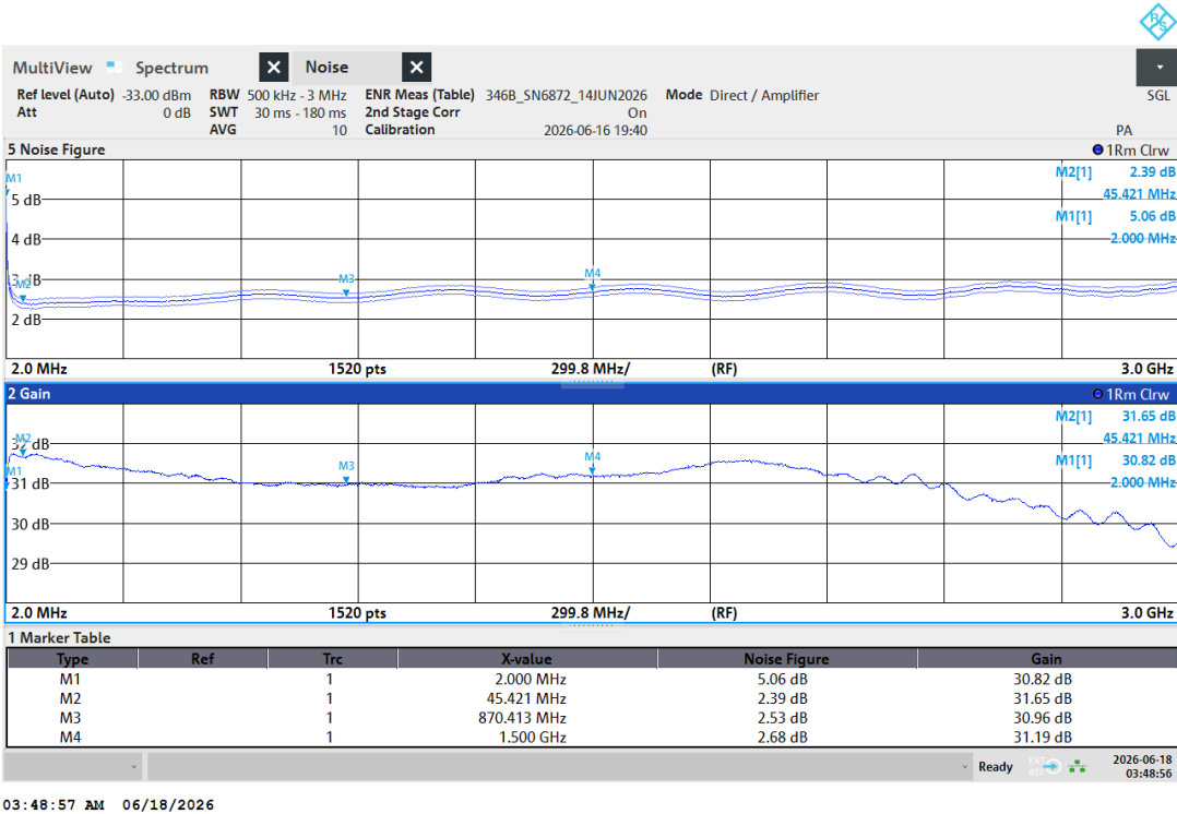
Figure 11.b ~ HP 8447A Modified (15 dB ENR)
