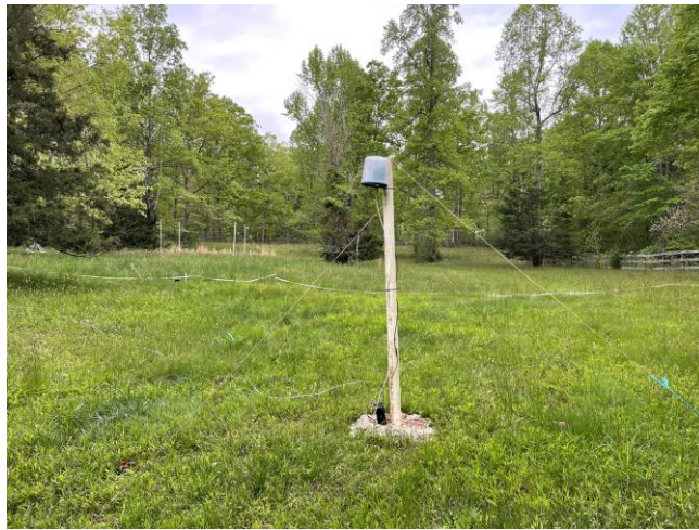
Figure 1, 38 MHz inverted “V” dipole with LNA enclosure over ground plane
