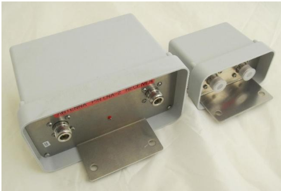
Figure 1.b ~ LNA-2 (left) and LNA-1 (right). Both LNAs have an antenna connector and receiver connector. The 12 Vdc powering voltage is fed through the receiver connector from a bias-tee near the receiver. The weatherproof cover is plastic while the mounting base/bracket is aluminum. A mast clamp is used with the amplifiers to attach to a mast immediately below the antenna.
