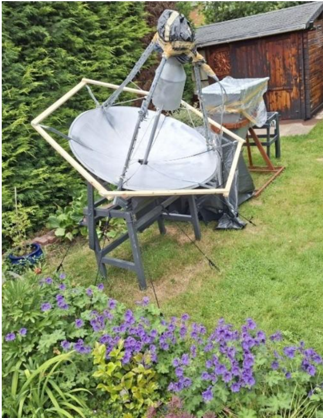
LRO-H2, 150cm Solar Cooker Petal Dish with bespoke Brian Coleman hydrogen line feed, and the start of the construction of surrounding mesh extension in an attempt to reduce ground spillover:
