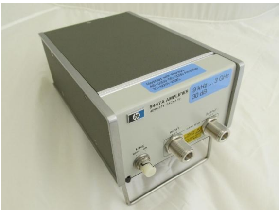
Figure 1.c ~ HP 8447A Modified. This is a lab amplifier and not intended for dedicated use with a receiver. This particular unit has been internally modified with a Wenteq ABL0300-00-3030 amplifier that replaces the original HP amplifier. The modification included replacing the original BNC-F connectors on the front panel with type N-F connectors as well as modifying the internal power supply for the lower voltage required by the Wenteq amplifier.
