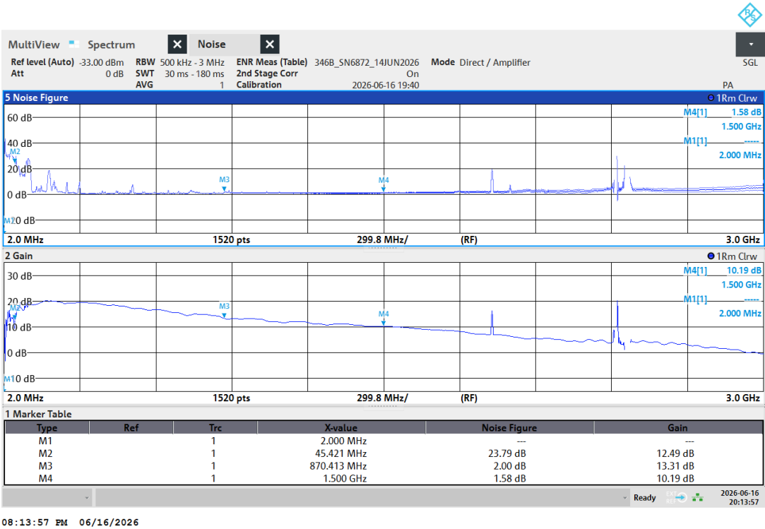
Figure 8.b ~ LNA-1 LNA (15 dB ENR): 2 – 3000 MHz
