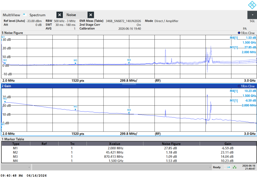
Figure 8.b ~ LNA-1 LNA (15 dB ENR): 2 – 3000 MHz
