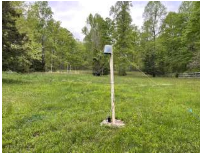
Figure 1, 38 MHz inverted “V” dipole with LNA enclosure over ground plane
