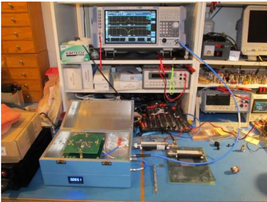
Figure 5.a ~ Foreground : NenuFAR LNA in test fixture before lid is closed and latched. The HP 346A noise source is connected with the HP 346B stands by. Background : FPL1003 analyzer.
