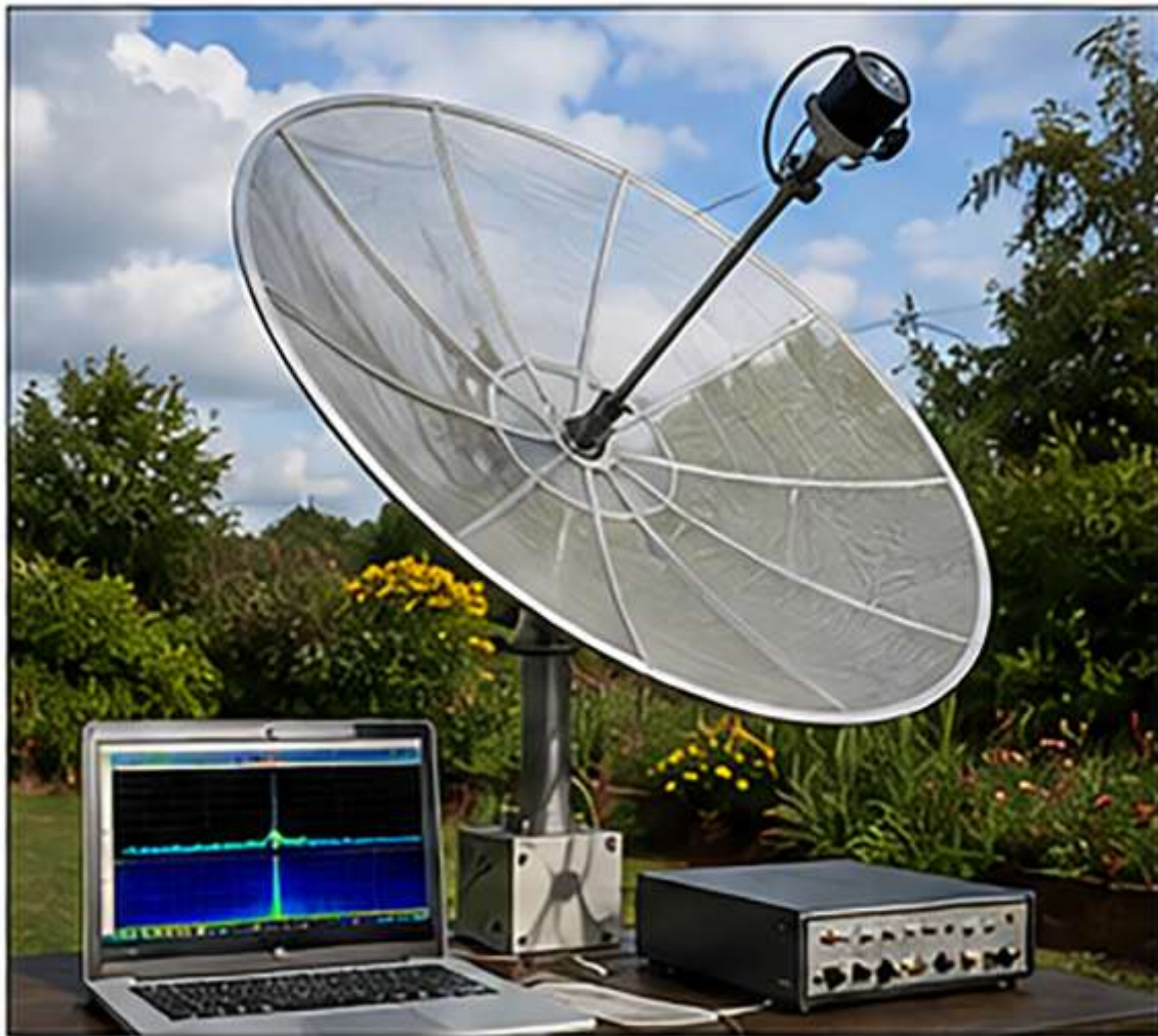
Figure 1. A typical Hydrogen Line observing station using an SDR receiver and parabolic dish antenna.
