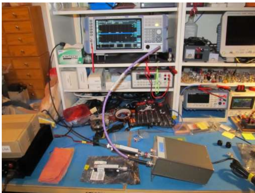
Figure 5.d ~ HP 8447A Modified showing HP 346A in use and HP 346B below.
