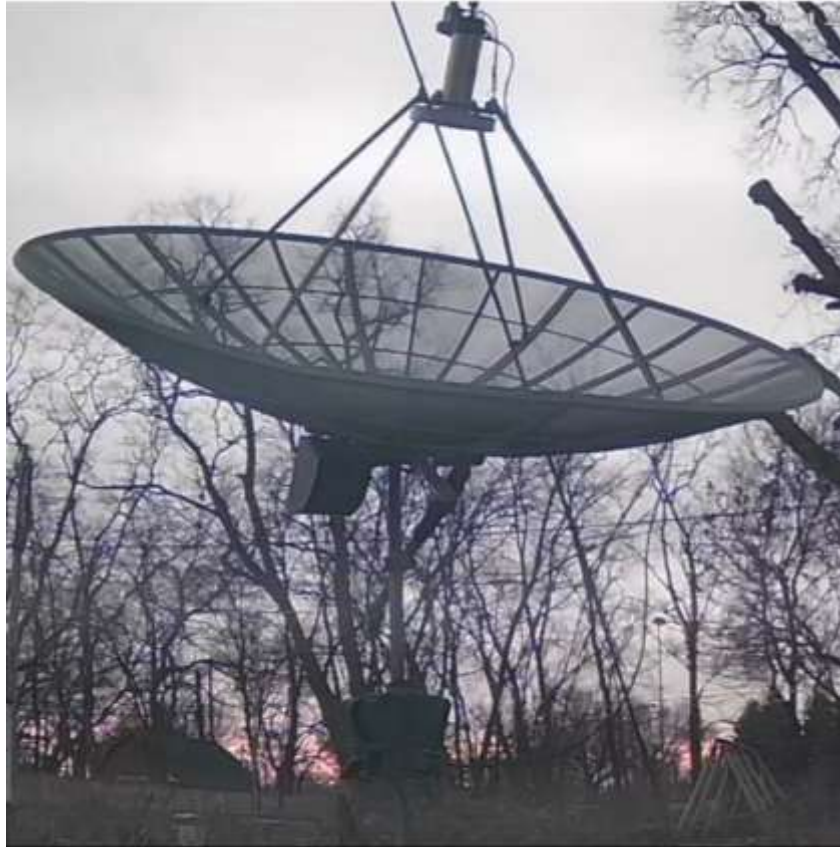
Figure 1. (a) Physical 4.5-meter mesh dish assembly and feed setup. (b) Control instrumentation station and processing suite.
