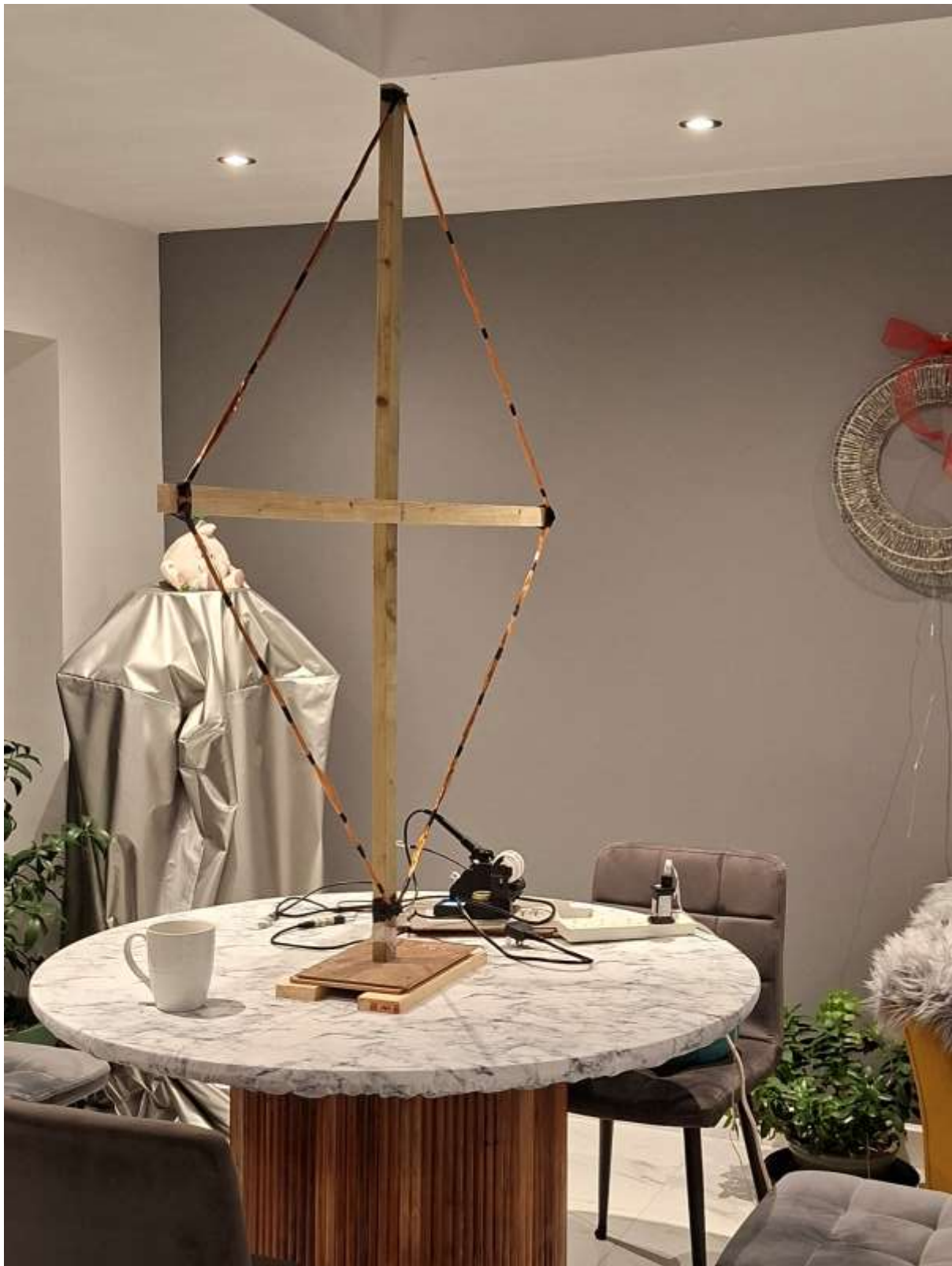
Photograph of the 134 cm square loop antenna showing wooden cross-frame support and perimeter winding. The loop is constructed from enameled copper wire wound around the
