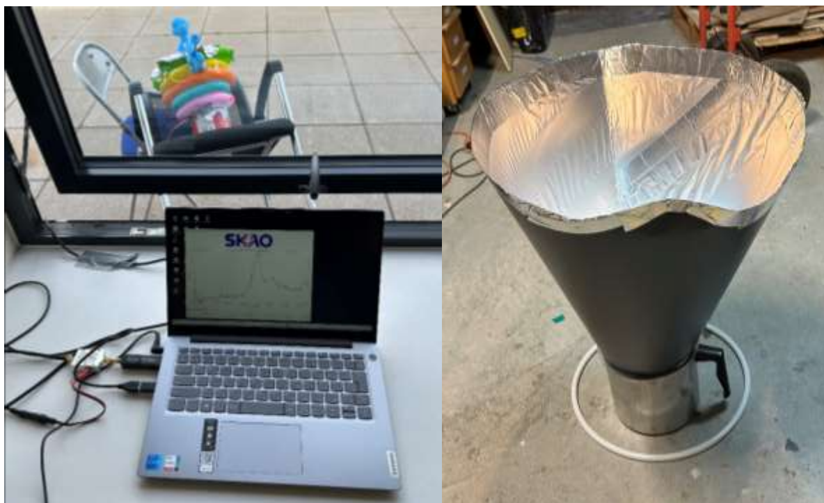
Figure 1: left: Dr. Shinichiro's hydrogen line demo at EUCARA. Right: transportable horn antenna built for hydrogen line demonstrations at the HTT 2025 star party.
