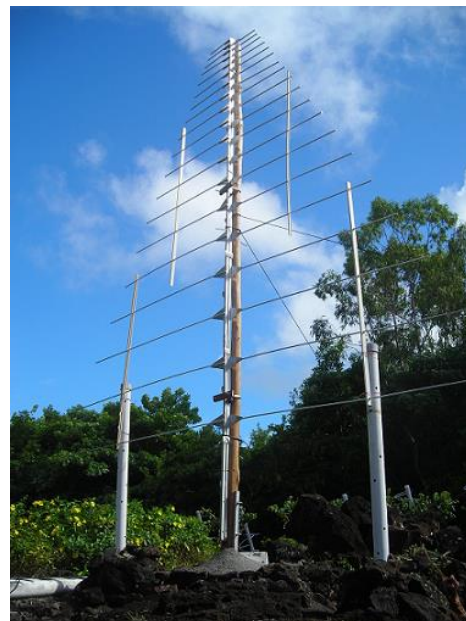
Self-manufactured LPDA, mounted on an old/dry Eucalyptus tree. Long dipoles were supported by plastic tubes from sanitary shop.
