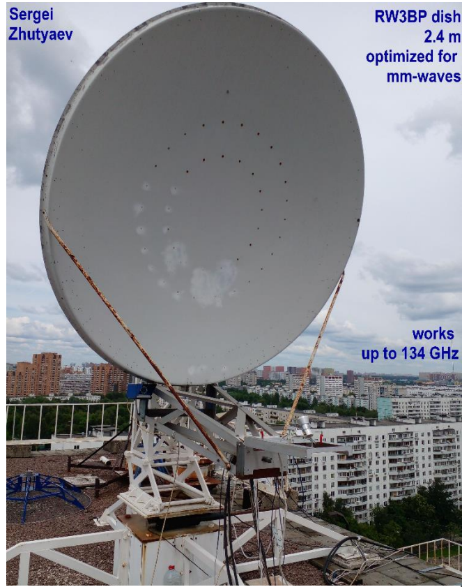
Figure 6. 2.4 m dish mounted on the roof of apartment building ( 55°46'00.5"N 37°49'25.8"E ) with 6.7 GHz RX downconverter at the focus. The dish was designed by Sergei Zhutyaev RW3BP for mm-waves initially.
