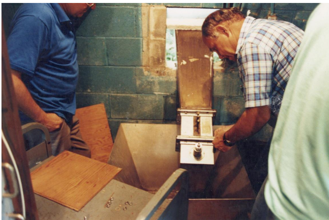
Jim Carroll N4CAE connects the waveguide to coax transition to the horn to attach his receiver.
