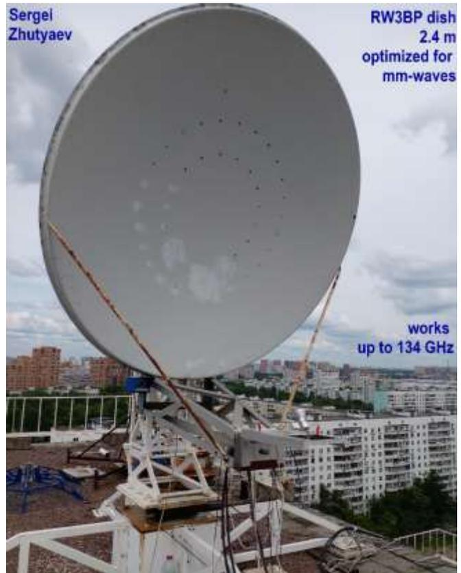
Figure 6. 2.4 m dish mounted on the roof of apartment building ([55°46'00.5"N 37°49'25.8"E](#)) with 6.7 GHz RX downconverter at the focus. The dish was designed by Sergei Zhutyayev RW3BP for mm-waves initially.
