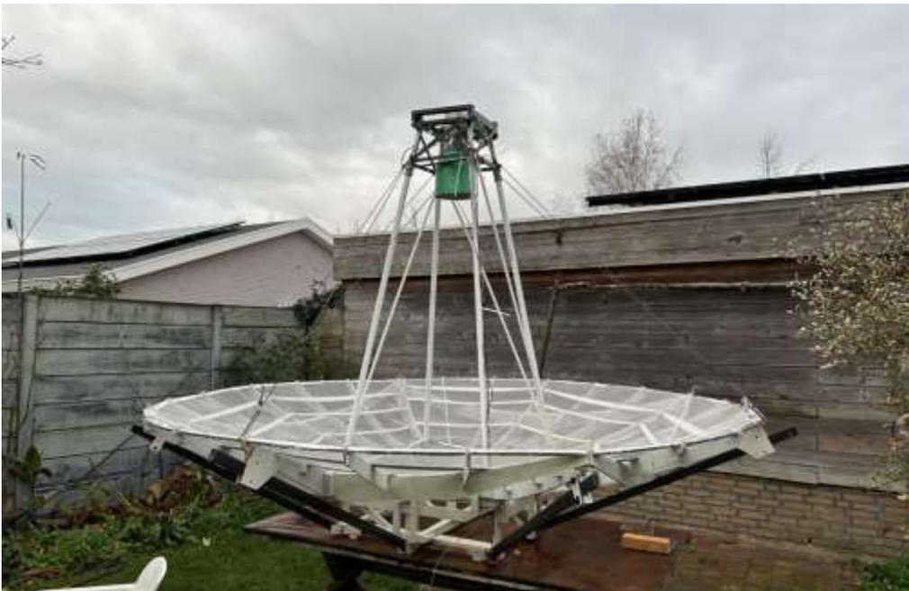
*Figure 8: the modular 3 metre dish.*
