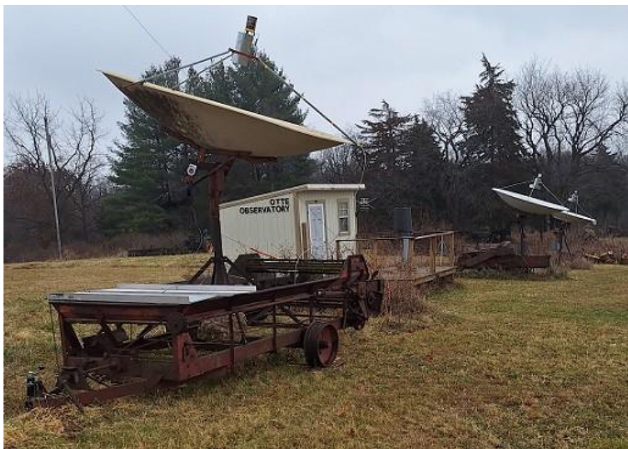
Image 1: Showing the 3 dishes spaced 10.6 M (1-2), 20M (2-3), and 31M (1-3) in an E-W line
