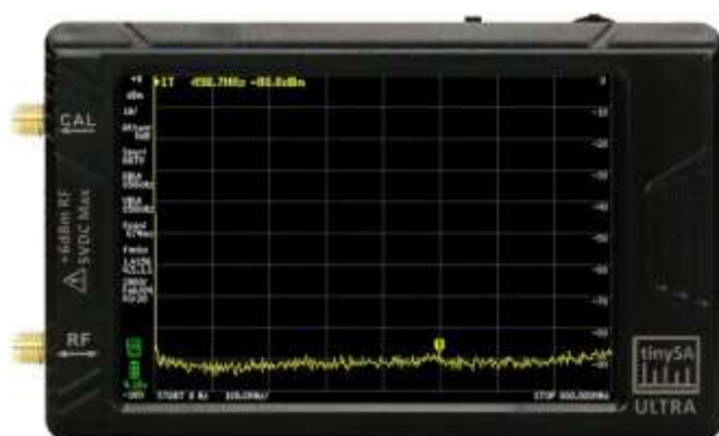
Figure 1 ~ TinySA Ultra. The touchscreen size is 4 inch diagonal with 480 x 320 pixel resolution. The spectrum analyzer RF input is the lower SMA connector on the left. The upper connector is for the signal generator RF output (primarily used for calibration). The On-Off power switch is on the top along with a jog switch for menu control. A USB-C connector for battery charging and connection to a PC, microSD memory card connector and earphone jack are on the bottom. The unit is based on the Silicon Labs Si4468 RF transceiver and STMicroelectronics STM32F302 processor ICs. Image source: https://www.tinysa.org/wiki/
