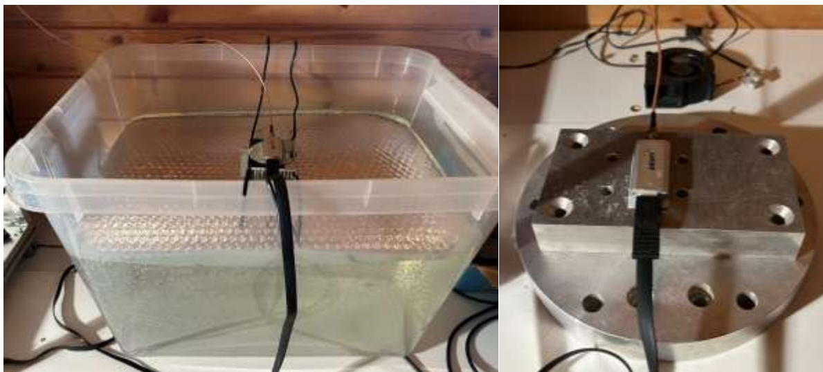
Figure 4: methods for thermally stabilizing the SDR. Left: using 50 litres of water as thermal mass; right: using aluminium blocks and a PC cooling fan. In both cases the SDR is attached to the heatsink with thermal paste to ensure optimal heat exchange.
