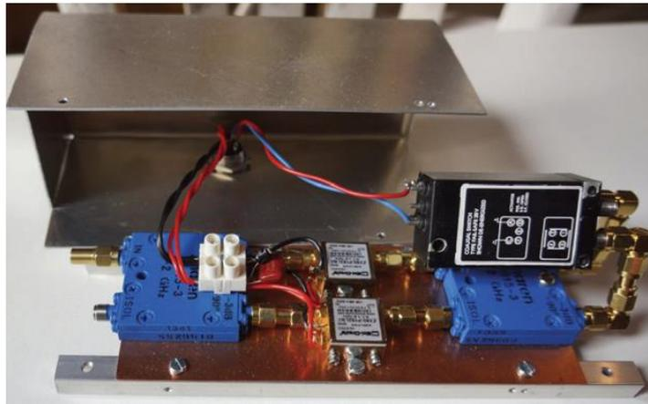
**Figure 5.** Hybrid LNA Correlation Receiver Section
