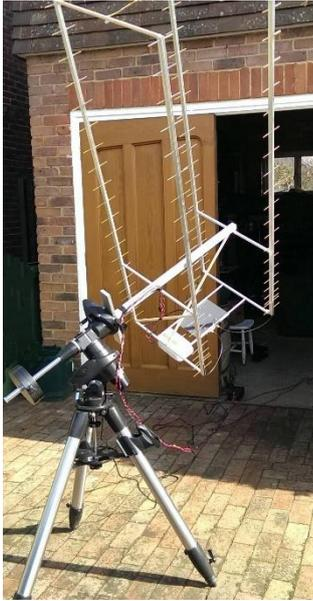
**Figure 4.** Hydrogen Line 22-element Quad Yagi Antenna
