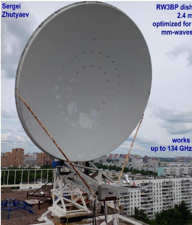
Figure 1. 2.4 m dish mounted on the roof of apartment building ([55°46'00.5"N 37°49'25.8"E](#)) with 6.7 GHz RX downconverter at the focus. The dish was designed by Sergei Zhutyayev RW3BP for mm-waves initially.
