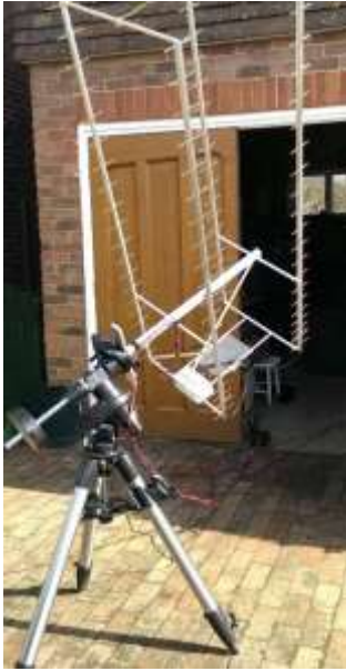
Figure 4. Hydrogen Line 22-element Quad Yagi Antenna
