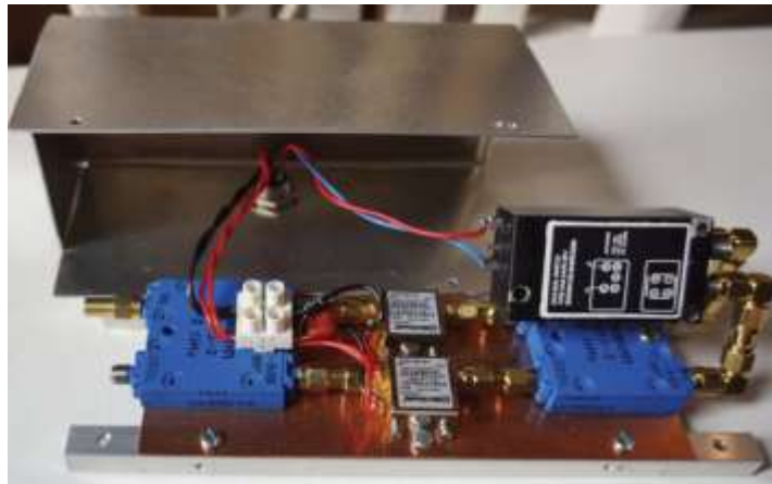
Figure 5. Hybrid LNA Correlation Receiver Section
