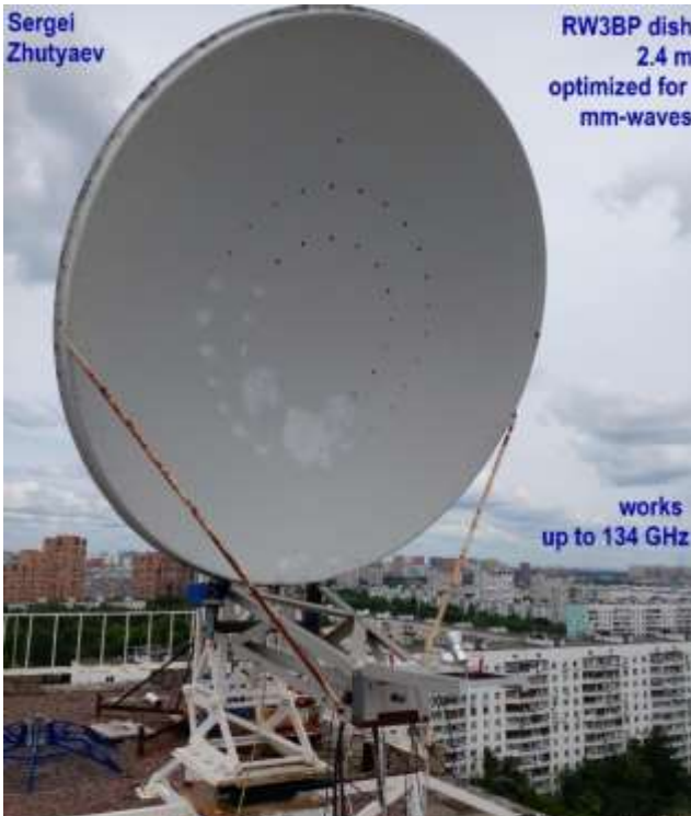
Figure 1. 2.4 m dish mounted on the roof of apartment building ( 55^\circ 46' 00.5'' N 37^\circ 49' 25.8'' E ) with 6.7 GHz RX downconverter at the focus. The dish was designed by Sergei Zhutyaev RW3BP for mm-waves initially.
