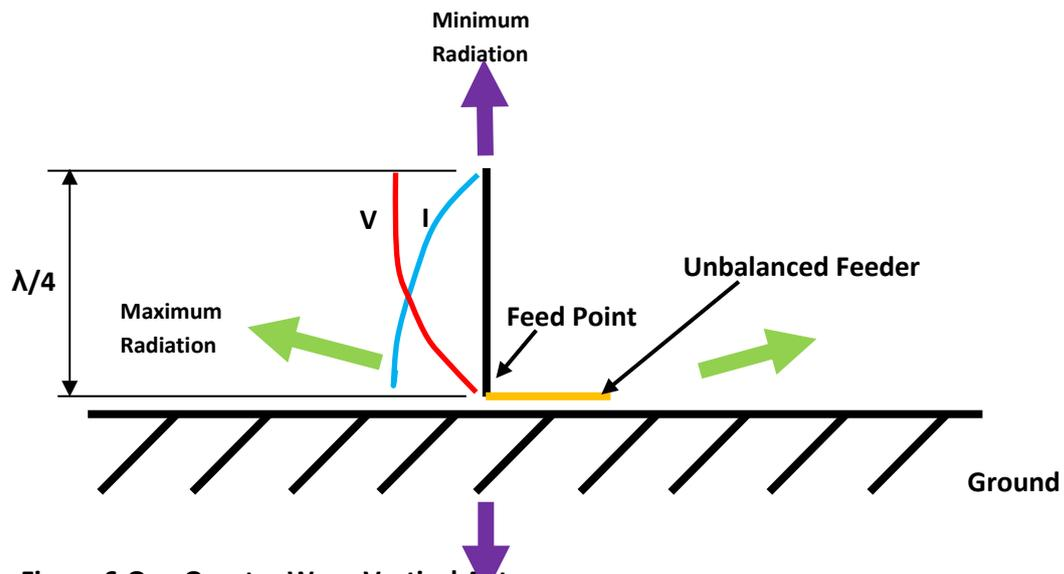
Figure 6: One Quarter Wave Vertical Antenna
