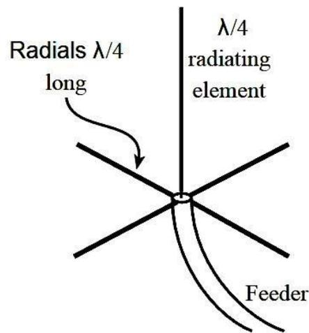
Figure 8. Example  $\lambda/4$  Ground plane Vertical Antenna
