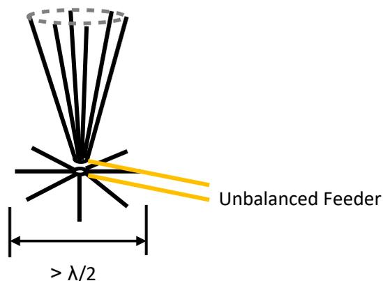
Figure 14. Monocone Antenna Using Radial Wires
