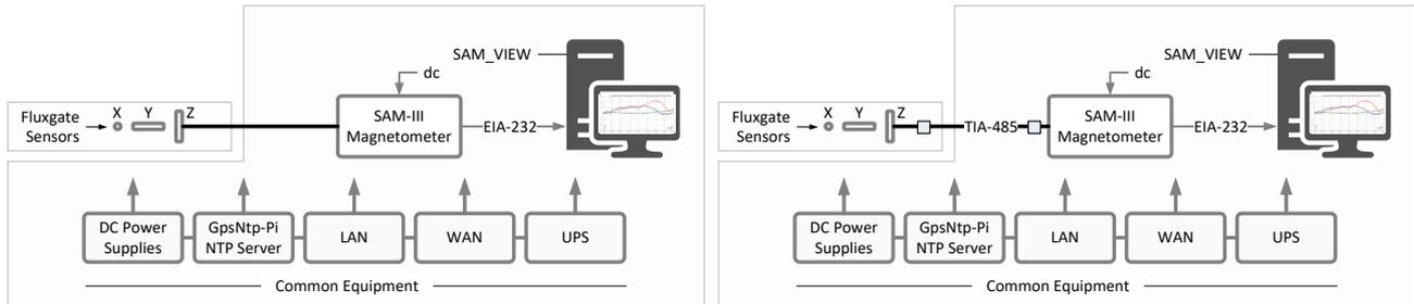
Figure 15 ~ SAM-III Magnetometer block diagrams for Anchorage (left) and HAARP (right). The two are operationally identical and differ only in a few technical details (see text).
