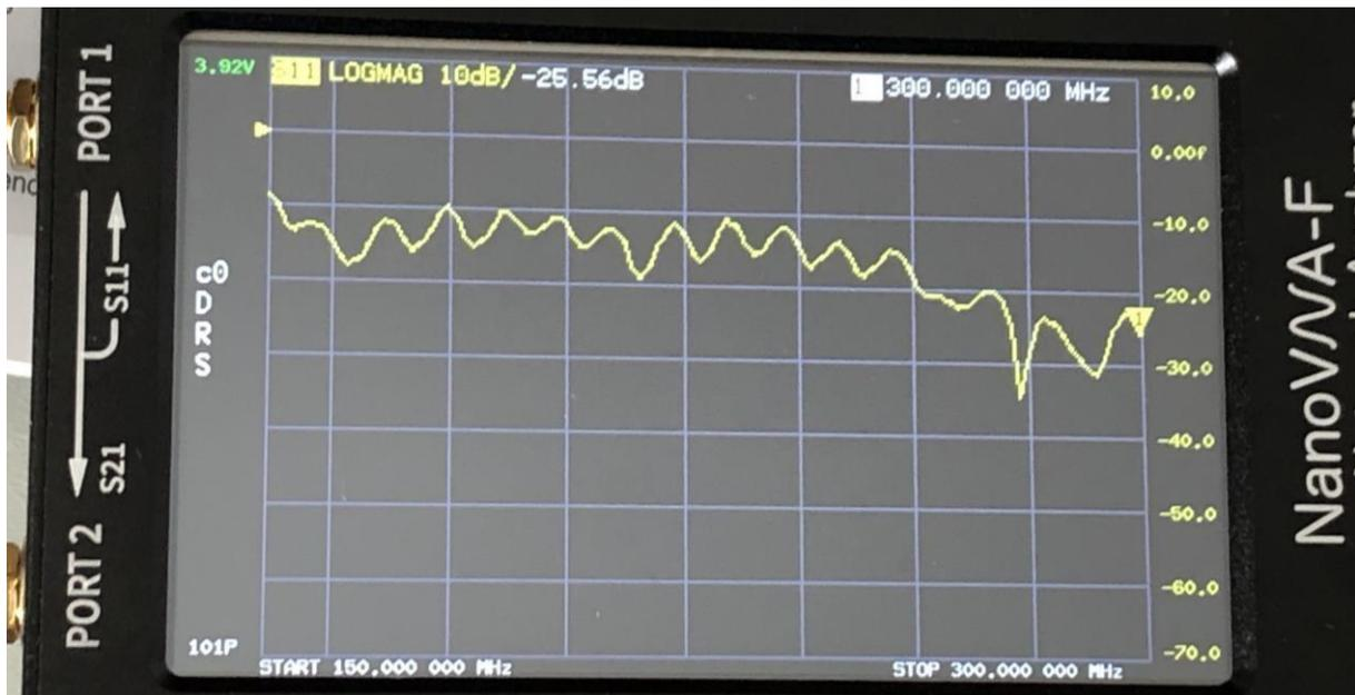
Figure 20. Discone Input Return Loss 150 to 300 MHz
