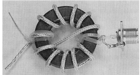
Figure 5. Balanced to Unbalanced Antenna Coupling
