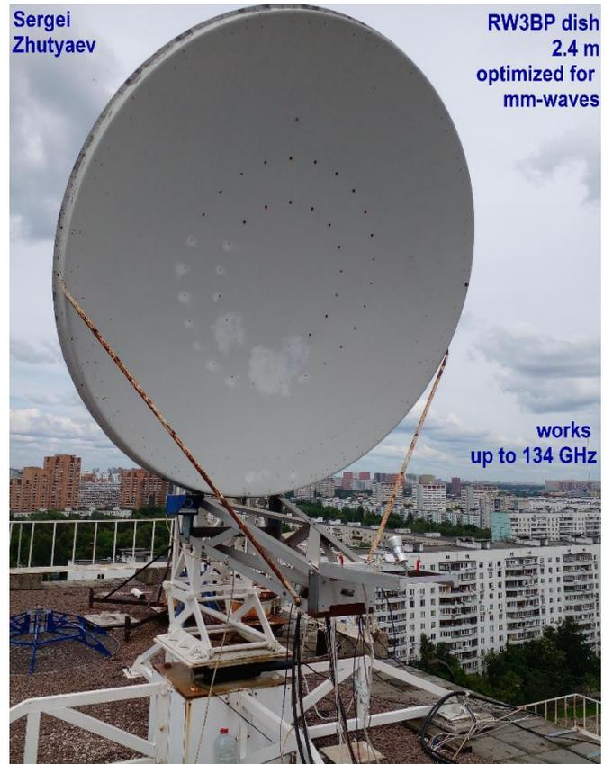
Figure 3. 2.4 m dish mounted on the roof of apartment building ([55°46'00.5"N 37°49'25.8"E](#)) with 6.7 GHz RX downconverter at the focus. The dish was designed by Sergei Zhutyaev RW3BP for mm-waves initially.
