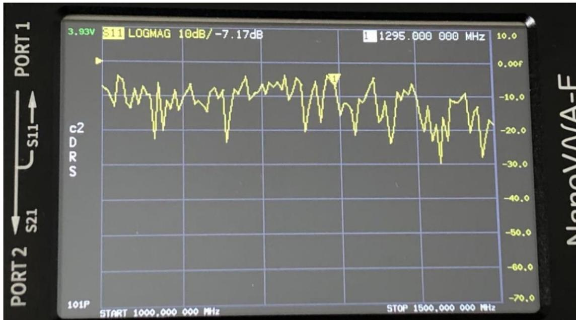
Figure 23. Discone Input Return Loss 1000 to 1500 MHz
