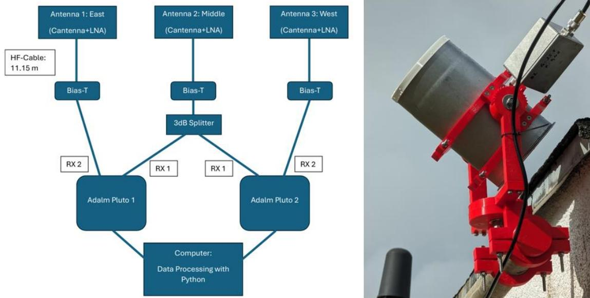
Figure 1: On the left, the interferometer setup is presented; on the right, one of the three antennas on its 3D printed mount can be seen.
