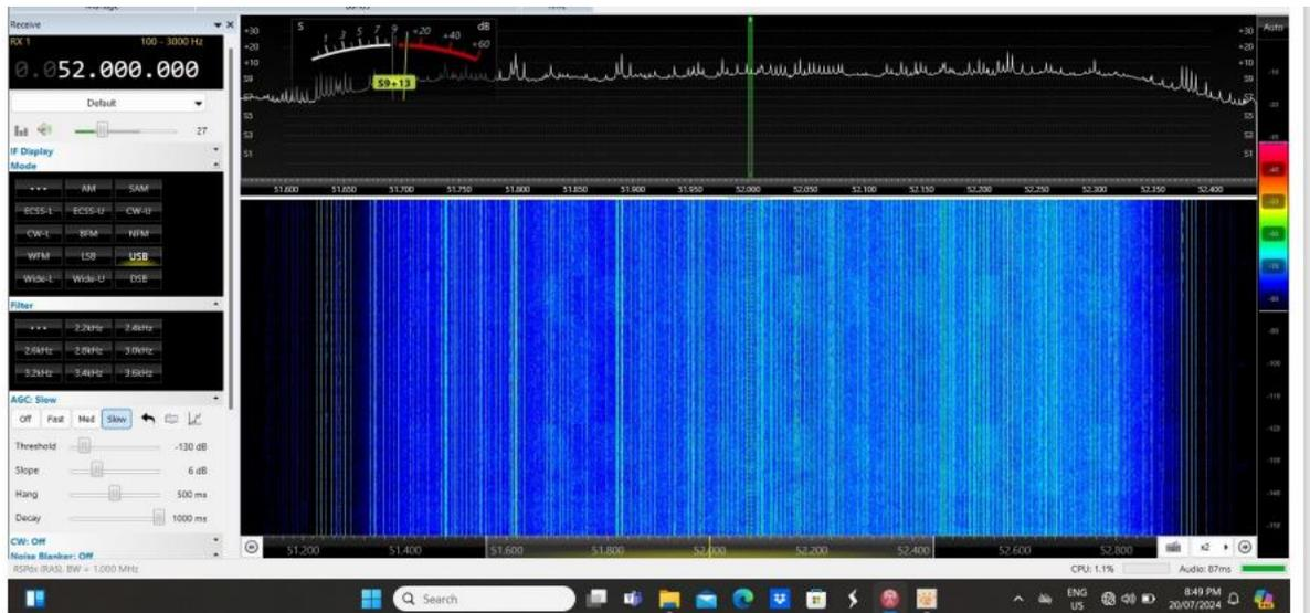
Figure 12. Screen Capture 52 MHz Band
