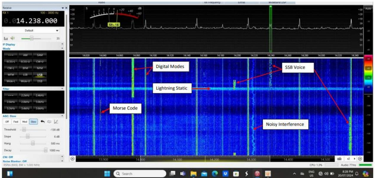
Figure 6. Screen Capture 14 MHz Band
