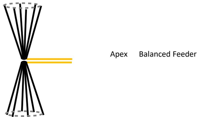
Figure 12. Bicone Antenna using Radials
