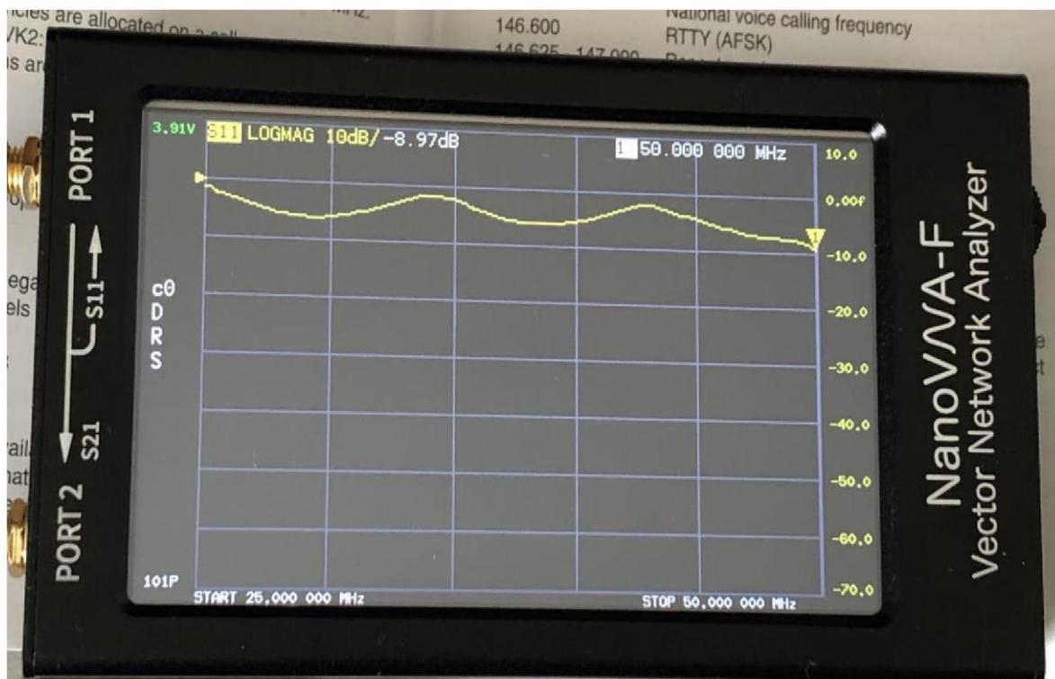
Figure 18. Discone Input Return Loss 25 to 50 MHz
