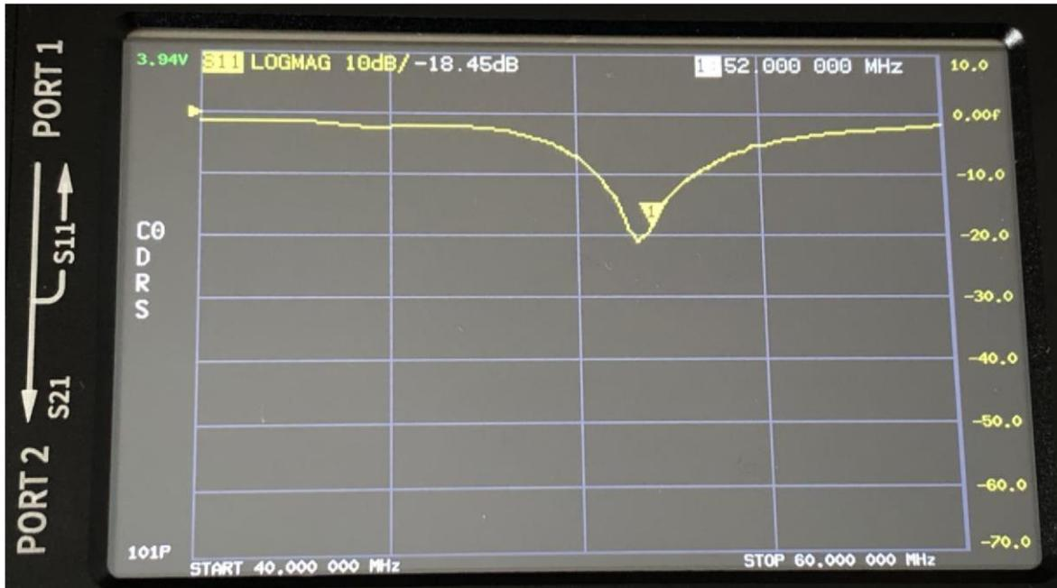
Figure 24. Discone Input Return Loss 6m band
