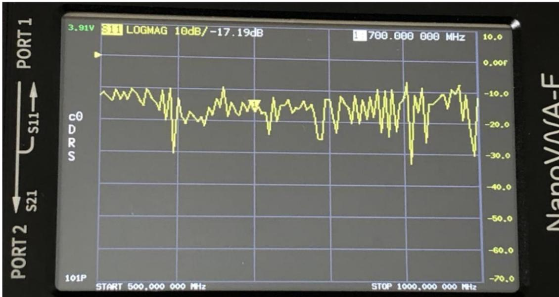
Figure 22. Discone Input Return Loss 500 to 1000 MHz
