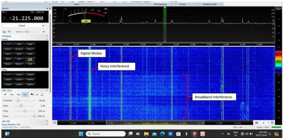
Figure 9. Screen Capture 21 MHz Band
