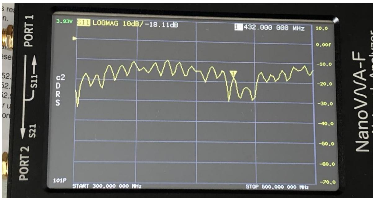
Figure 21. Discone Input Return Loss 300 to 500 MHz
