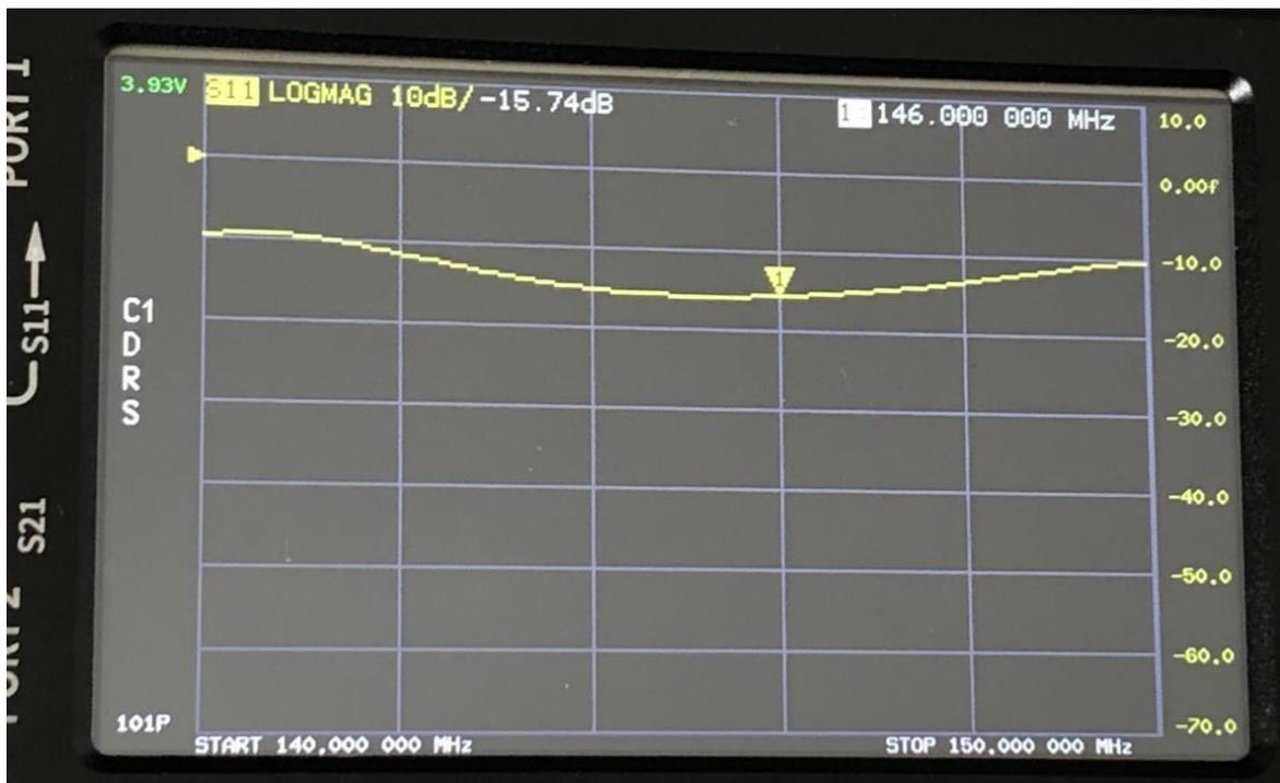
Figure 25. Discone Input Return Loss 2m band
