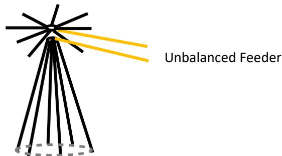
Figure 15. Inverted Monocone Antenna Using Radial Wires
