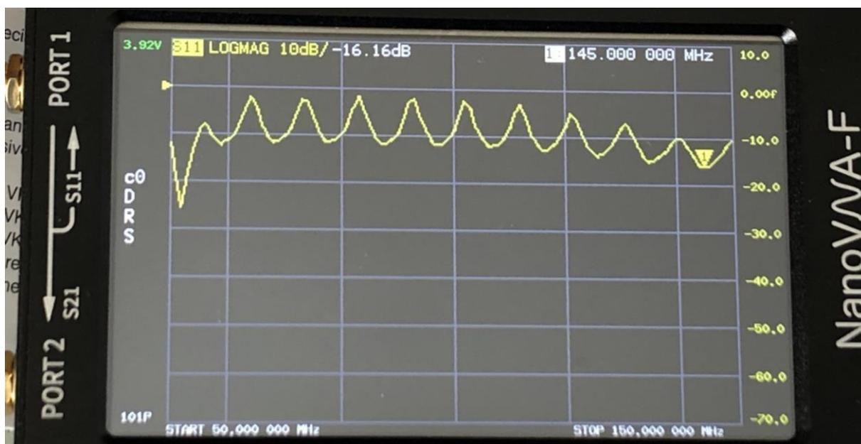
Figure 19. Discone Input Return Loss 50 to 150 MHz
