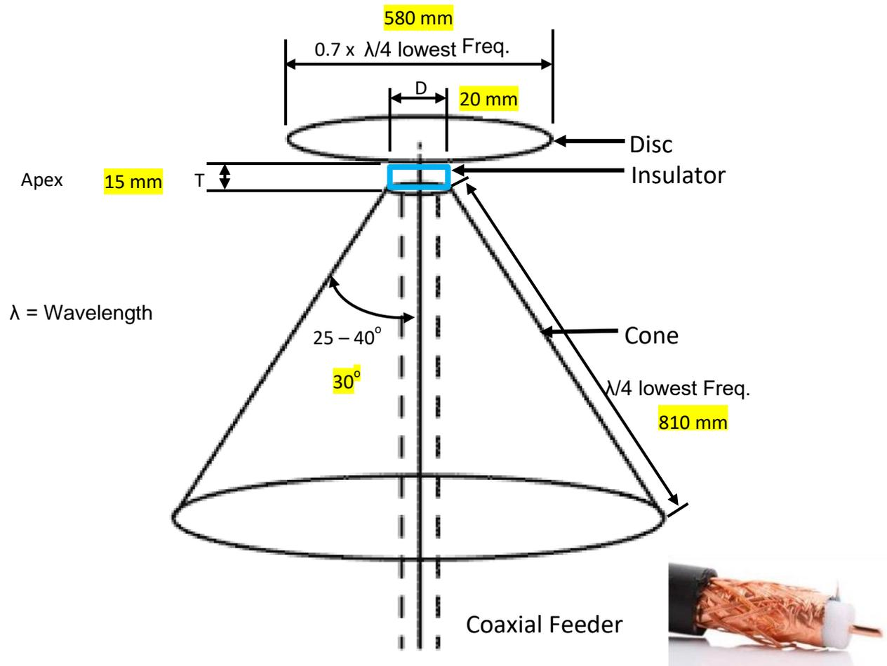
Figure 16. Discone Antenna Configuration
