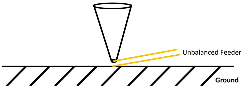
Figure 13. Monocone Antenna
