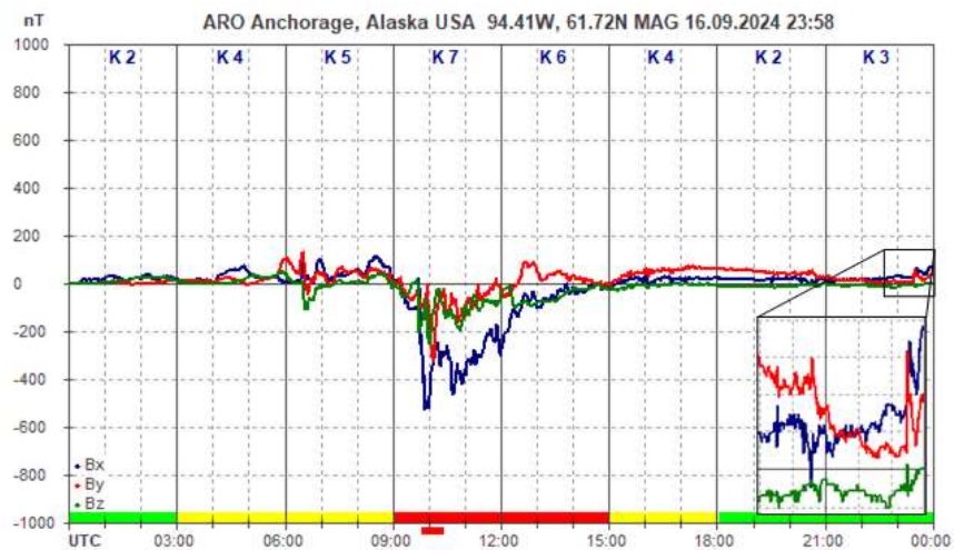
Figure 14.a ~ Anchorage magnetogram for 16 September annotated with the last three hours of the UTC day zoomed-in. All three components show evidence of the impulse (near right edge), including about 15 nT in the vertical component Bz. The sudden impulse amplitude at Anchorage was approximately 63 nT. Note the bay seen in the inset in the east-west component (By, red trace) during the 3-hour period leading up to the Sudden Impulse.
