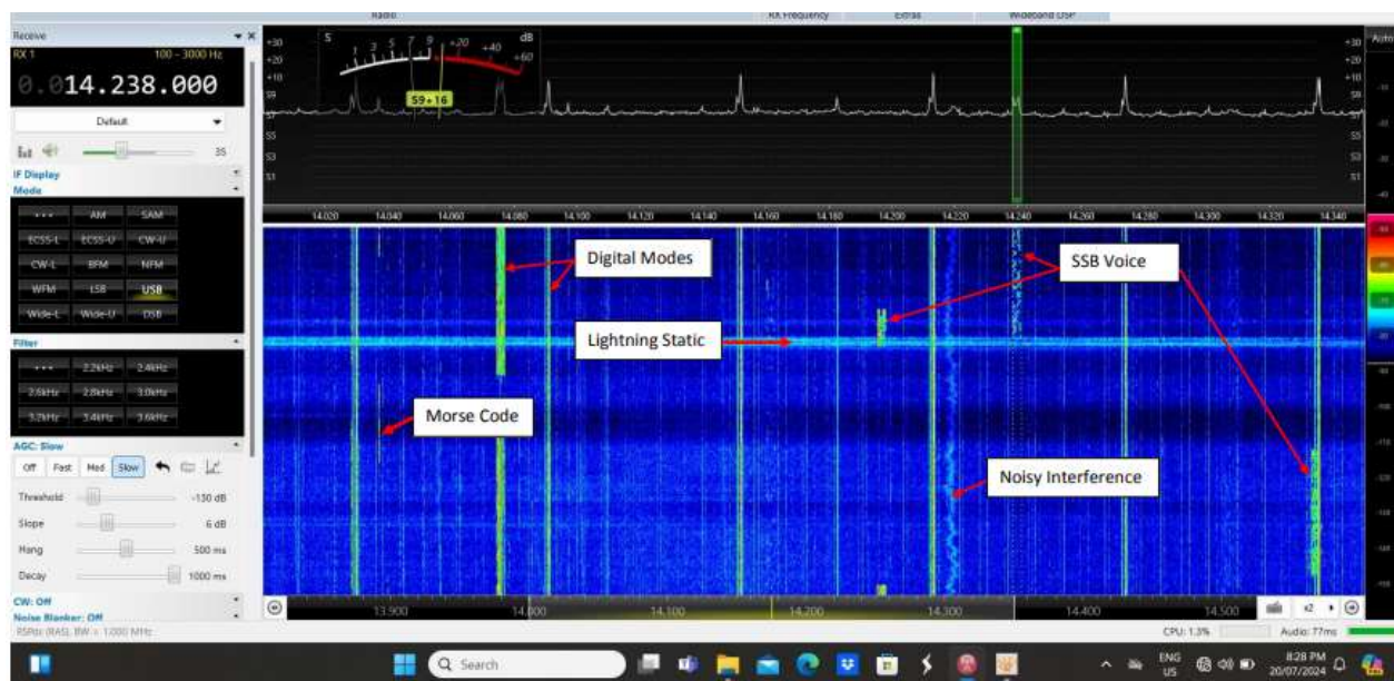
Figure 6. Screen Capture 14 MHz Band
