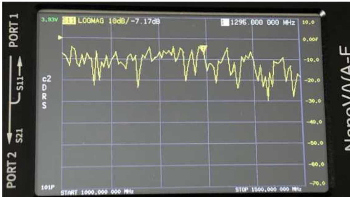
Figure 23. Discone Input Return Loss 1000 to 1500 MHz
