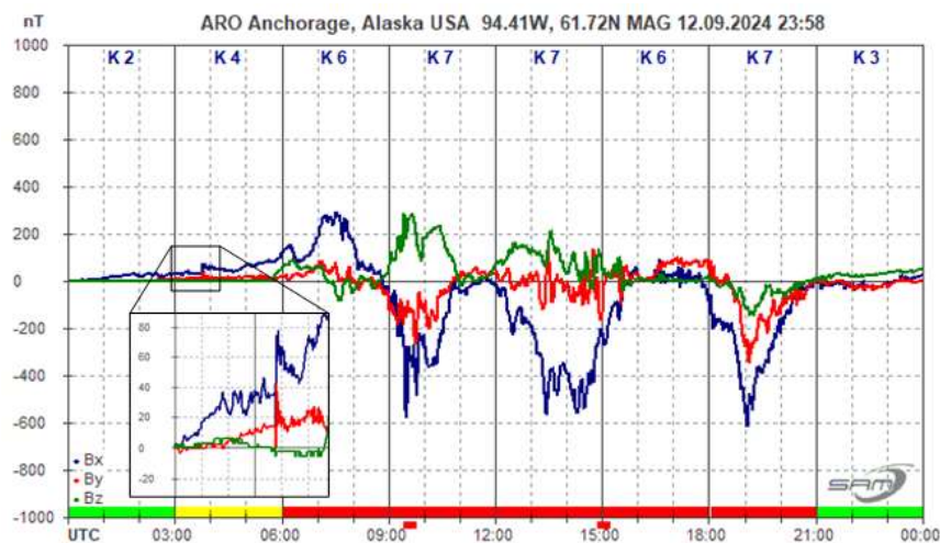
Figure 13.a ~ Anchorage magnetogram for 12 September. The vertical autoscale function of the SAM_VIEW software stepped to 1000 nT due to the high magnetic flux density at about 0930 following the Sudden Impulse. The impulse was almost invisible at this scale so the time from about 0300 to 0415 has been expanded in the inset to show more detail. The sudden impulse amplitude at Anchorage (vector sum of B_x and B_y ) was approximately 76 nT.
