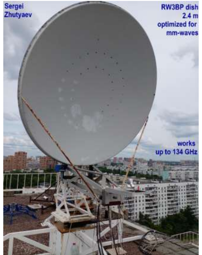
Figure 3. 2.4 m dish mounted on the roof of apartment building ( 55°46'00.5"N 37°49'25.8"E ) with 6.7 GHz RX downconverter at the focus. The dish was designed by Sergei Zhutyaev RW3BP for mm-waves initially.
