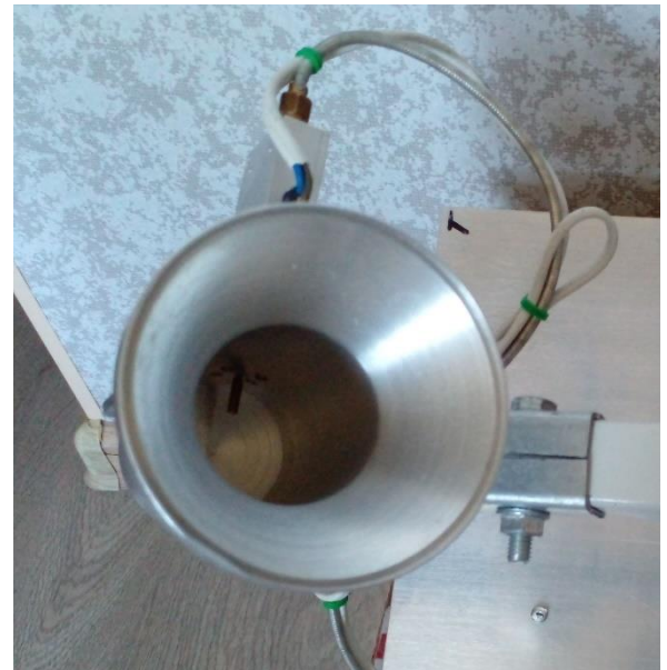
Figure 9. The feedhorn, looking inside.
