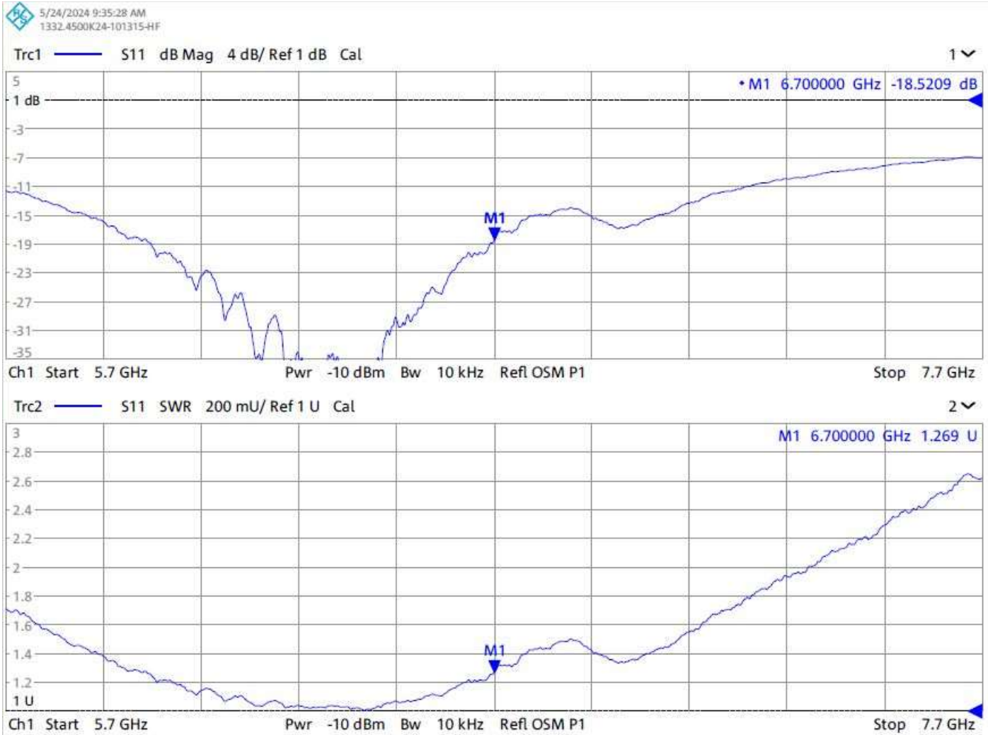
Figure 12. Measured data for reflections of the feedhorn at 6.7 GHz (R&S ZNA)
