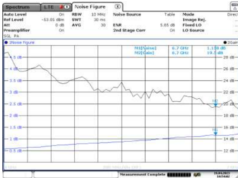
Figure 7. Measured Noise Figure and operating gain of LNA (R&S FSV, Noise Figure options, the noise head – Noisecom NC346A precision).
