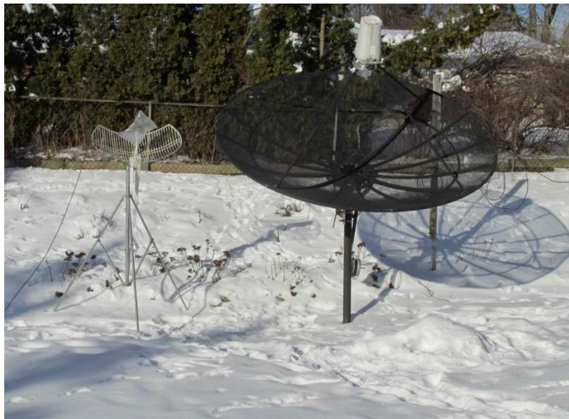
Figure 1. Interferometer Antennas
