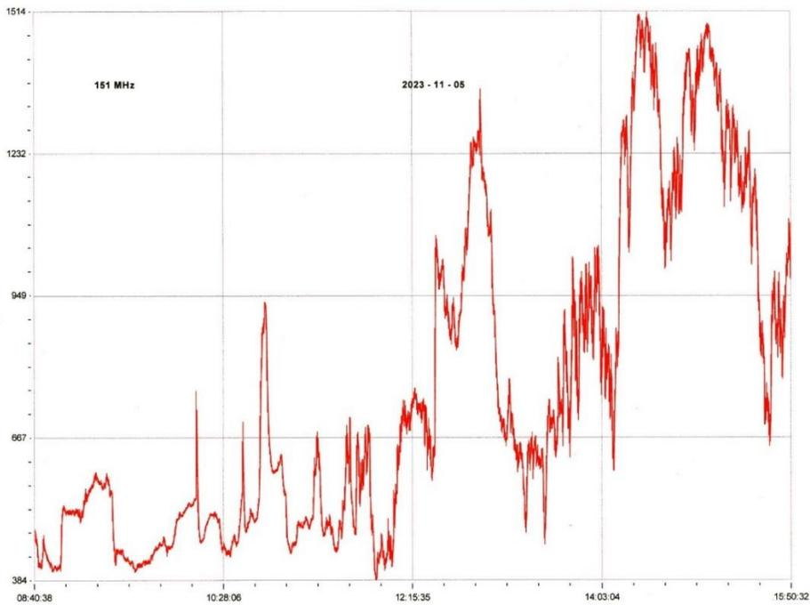
Colin Clements recorded some significant 151MHz solar noise during the strong flares on the 2<sup>nd</sup> and 5<sup>th</sup>. The aerial is now loft mounted and horizontally polarised, which seems to give a wider beam width for a fixed azimuth aerial. It is tricky to identify individual flares, as there were also plenty of smaller events that we did not record.
