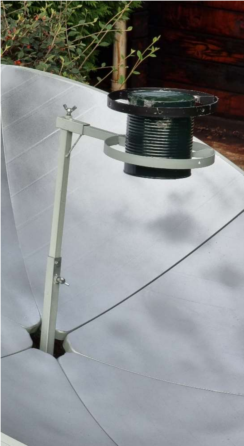
The photograph below shows the cantenna mounted in the new arrangement that is now used in the finished telescope.
