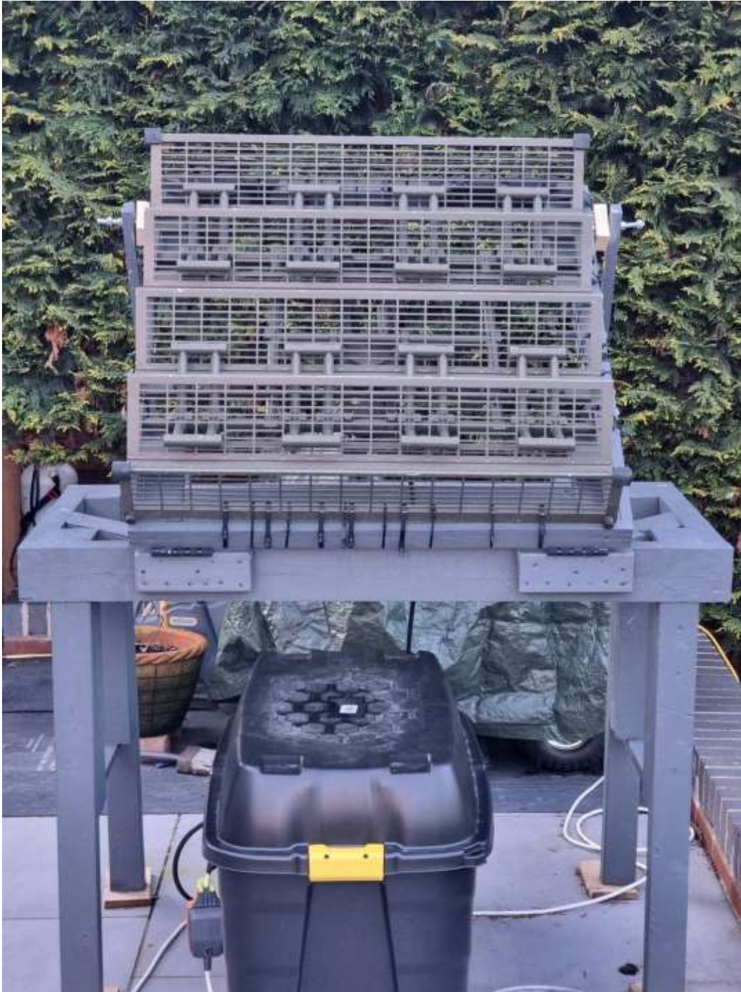
Ptarmigan Triffid Band 3 Ex-Military Dipole Array (below):
