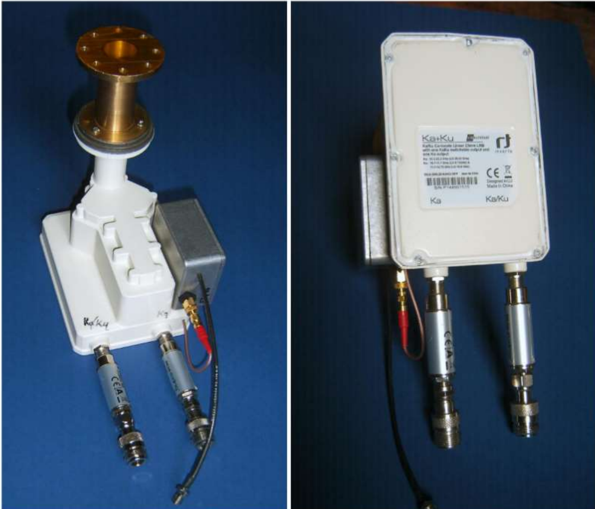
Figure 2: Ku- Ka band LNA with modification
