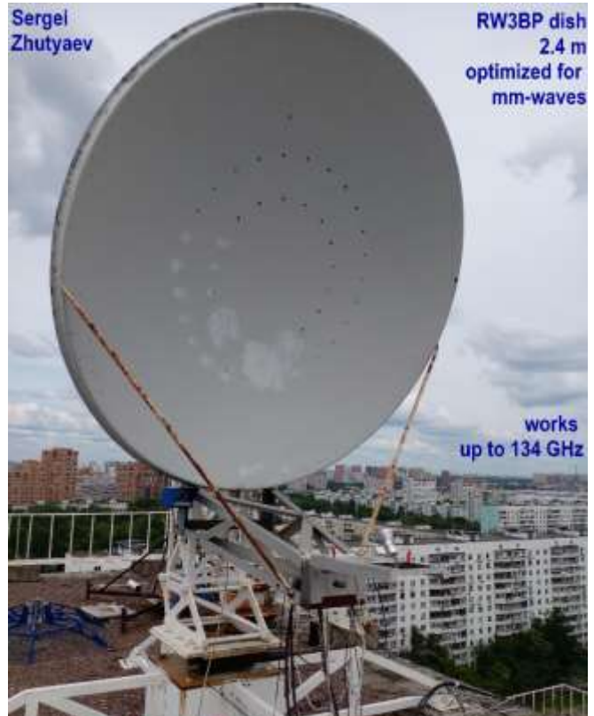
Figure 7. 2.4 m dish mounted on the roof of apartment building ( 55°46'00.5"N 37°49'25.8"E ) with 6.7 GHz RX downconverter at the focus. The dish was designed by Sergei Zhutyaev RW3BP for mm-waves initially.
