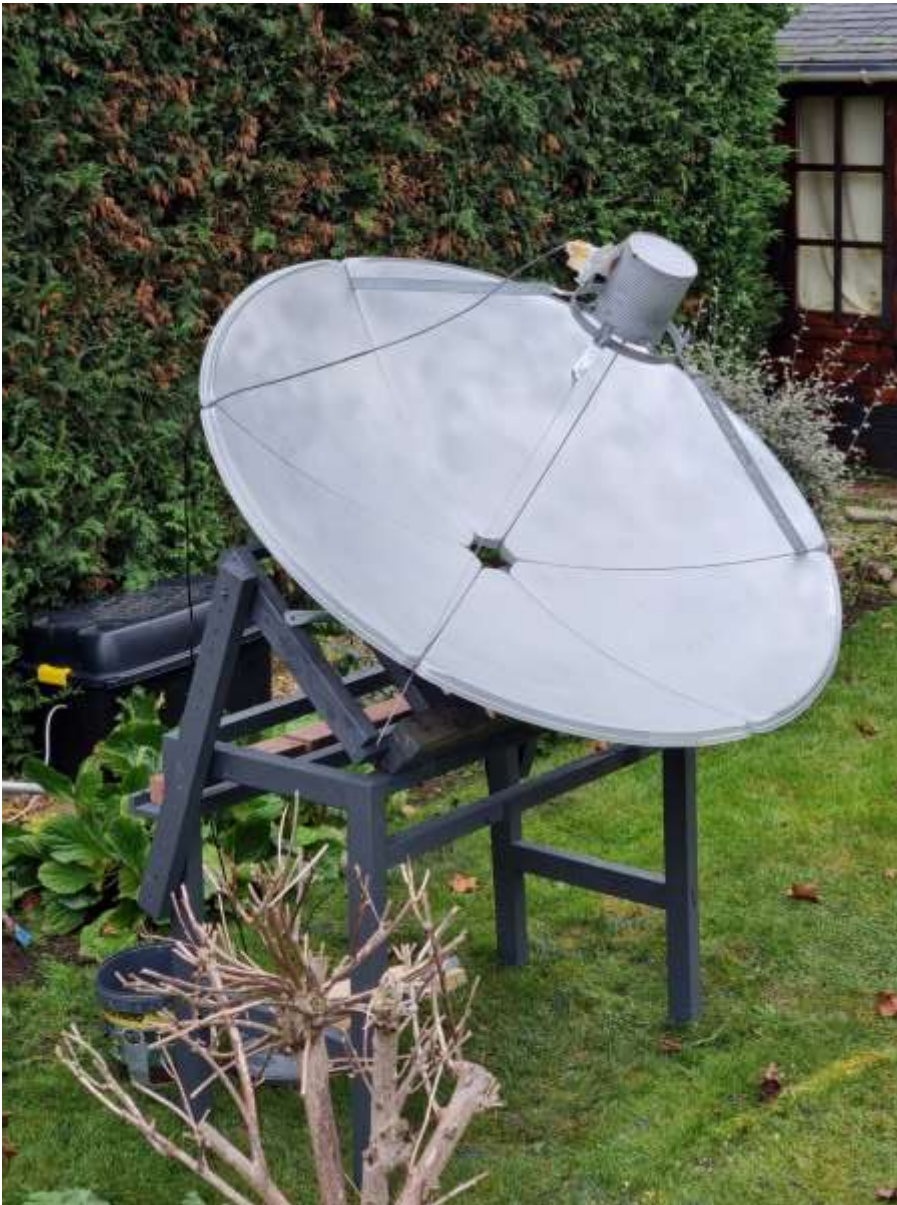
The cantenna I build showing the monopole inside made from a paper clip (below).
