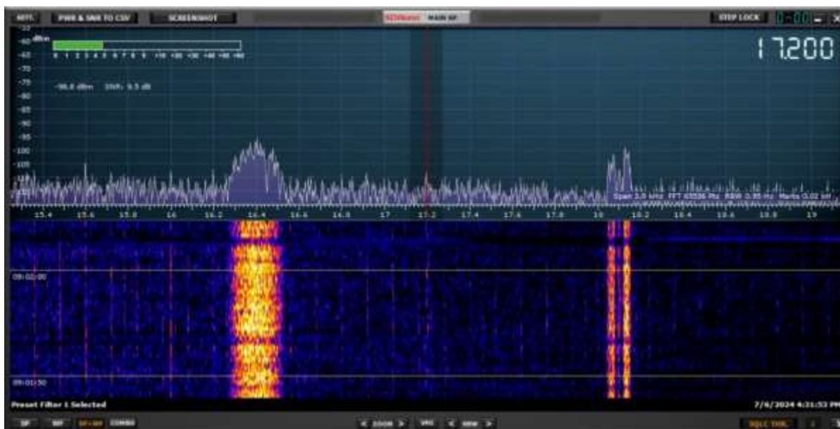
Figure 2.a ~ Waterfall spectra from 15.3 to 19.1 kHz with the SAQ signal at 17.2 kHz in the middle. Relative received signal power level is shown in dB on the left-vertical scale and frequency in kHz is shown along the middle-horizontal scale. The signal is very weak and indiscernible in the spectra but visible in the waterfall. The vertical lines in the waterfall are powerline harmonics at 120 Hz intervals. The brighter signal on the left is the Norwegian VLF station JXN at 16.4 kHz and the two signals to the right centered on 18.1 kHz are thought to be a Russian VLF station.
