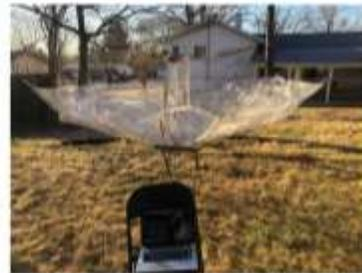
Finally Settled on "Faraday Fabric" with a window screening ground noise shield
