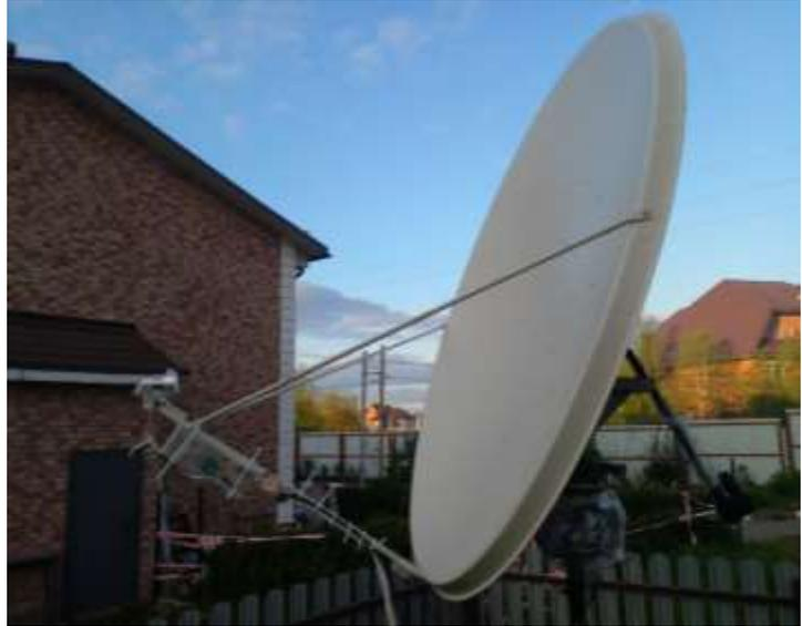
Figure 2. Methanol maser telescope 6.7 GHz.
