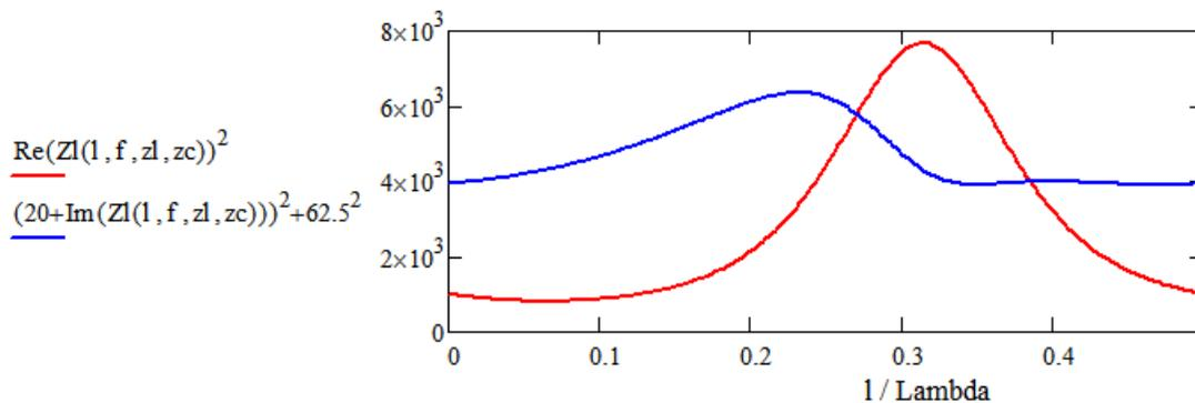
**Figure 7.** Confirmation of Optimum Transmission Line Lengths.
