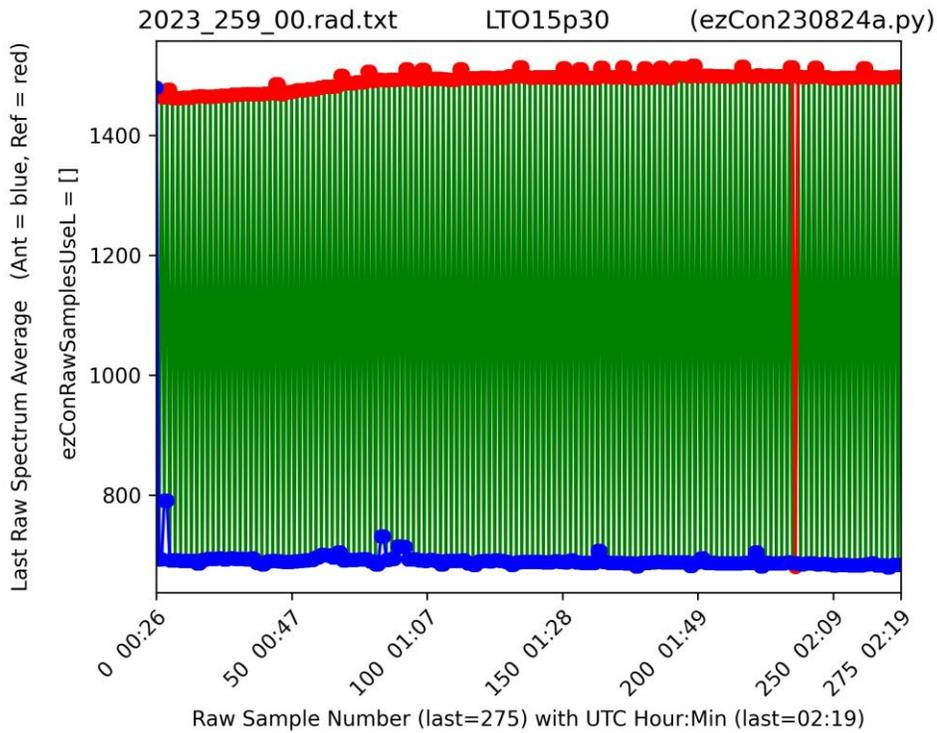
*This is an image showing how the antenna switches back and forth from looking at the sky(red) to looking at itself(blue). The red line indicates a machine error that will need to be cleaned later in the data refinement process.*
