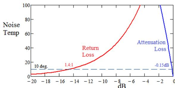
Figure 1. Attenuation and Mismatch (Return Loss) Contribution to  $T_{sys}$  Noise Temperature
