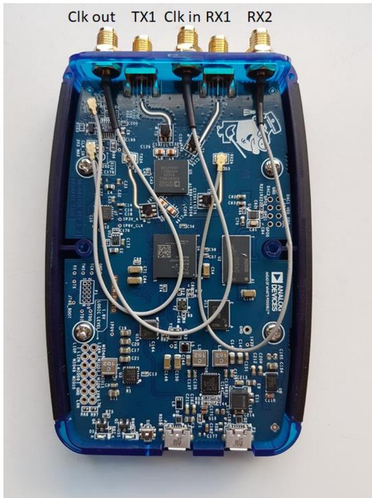
Figure 1: Modified ADALM Pluto (Rev. C board)
