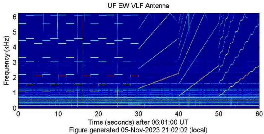
Figure 4 ~ HAARP induced ULF and VLF emissions received at Chistochina about 30 km northeast of HAARP on 5 November from a similar experiment. Acknowledgements: Robert Moore – University of Florida for ELF Receiver & Mark Golkowski – University of Colorado for the experiment sequence
