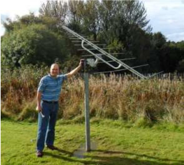
Figure 16 ~ Log periodic dipole array antenna (LPDA) mounted on a mast with a rotator and low noise amplifier. The 21-element Creative Design CLP5130-1N antenna frequency range is 50 to 1300 MHz and its free space gain is 6 to 8 dB. This antenna installation has a fixed elevation but can be turned to any hour angle with the rotator. The low noise amplifier has a noise figure of about 1.0 dB and a gain of about 20 dB. Setup at University of Glasgow, UK. Image ©2012 C. Monstein.
