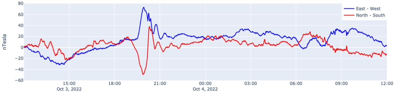
This recording from the 3<sup>rd</sup> and 4<sup>th</sup> by Nick Quinn shows a strong pulse around 20UT. It does not seem to be a CME impact, so is probably a shock in the solar wind. Recordings by Roger Blackwell show strong solar wind disturbances continuing on the 4<sup>th</sup>, 5<sup>th</sup> and 6<sup>th</sup>:
