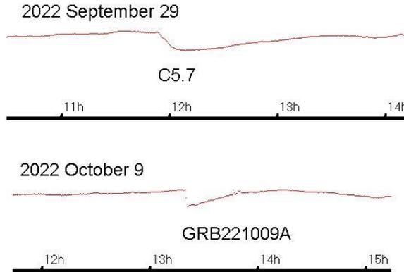
My own recording of the resulting SID compares in size to that of an ordinary C5.7 flare from last month, but has very sharp start and peak times. It looks more like a transmitter effect, but as it was also recorded on other signals then it must be from the GRB. There is a report on the qsl.net web site of a GRB detection on 2003 /03/29 using a 75kHz signal, although with a very short spike shaped SID.
