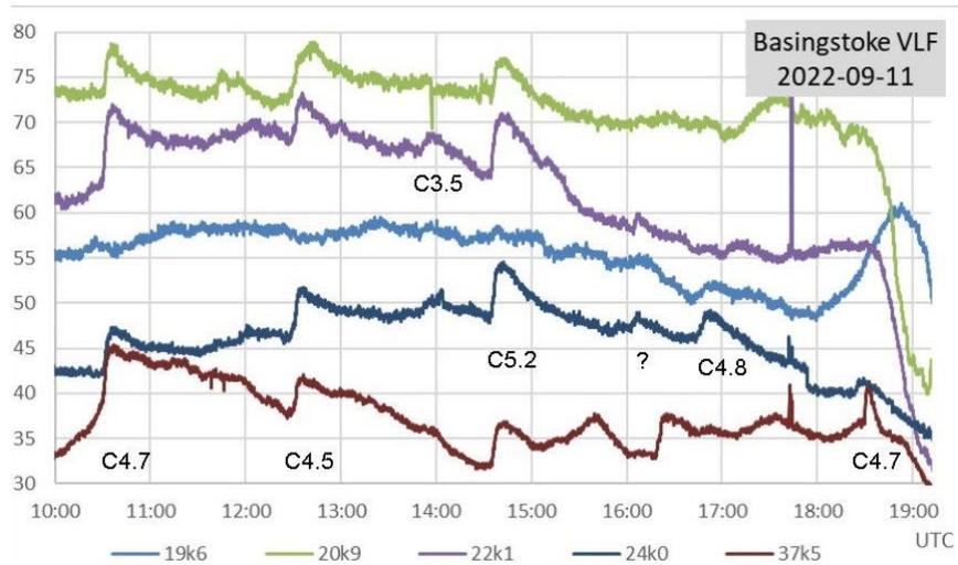
Paul Hyde's recording from the 11<sup>th</sup> shows a better spaced series of flares, although with some noise present. The spikes seen around 17:50 are from an induction hob, and so easy to eliminate. They can also be seen in the recording from the 16<sup>th</sup> shown previously.
