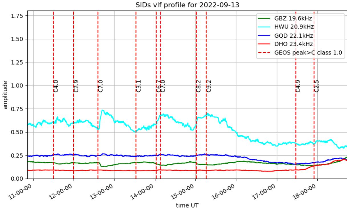
This recording by Mark Prescott on the 13<sup>th</sup> shows how the many overlapping flares have made analysis very difficult. The C7.0 flare at 12:40 produced a very clear SID, while those through the afternoon have become much less clear.
