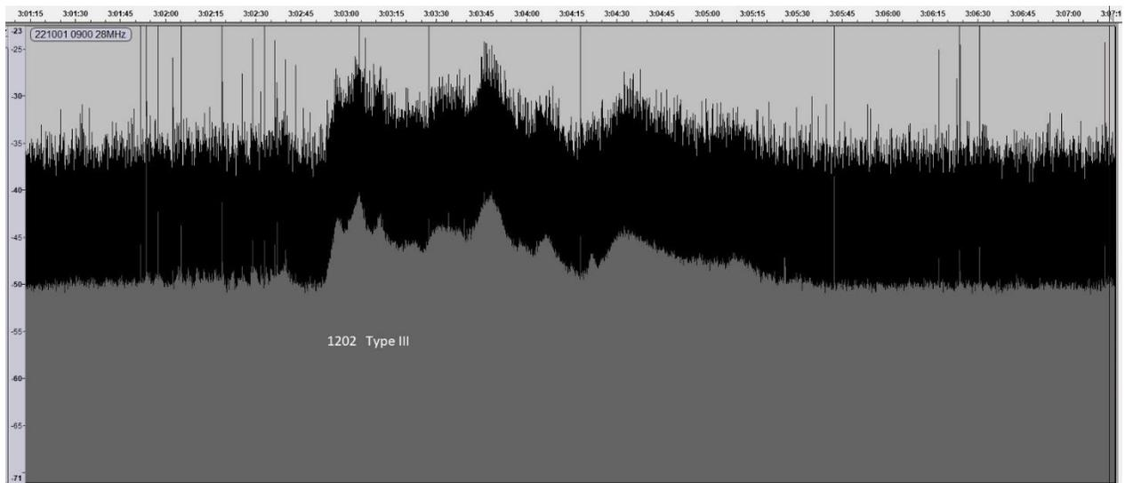
We did not record a SID at this time, but the SWPC bulletin does list a C3.5 flare starting at 11:00 with a peak at 13:00. Looking at the GOES X-ray data does show a smaller peak of about C2 at 12:00, confirming the link. It was a fairly weak burst of about 10db amplitude, lasting five minutes. The sun is now too low in the sky for Colin Clements to record VHF/UHF emissions.
