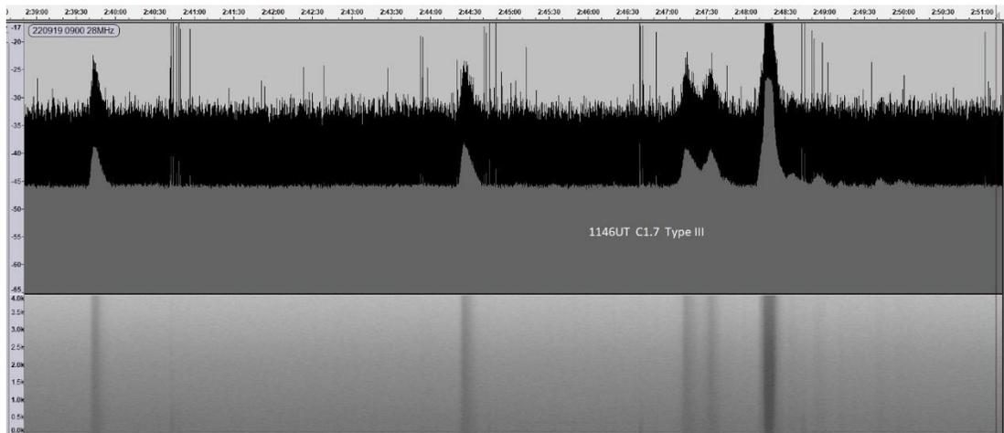
This 28MHz type III signal is from the 19<sup>th</sup>, peaking about 20dB above the background at 11:46 on the 19<sup>th</sup>. Its timing matches a C1.7 flare, although we did not record a SID from it.
