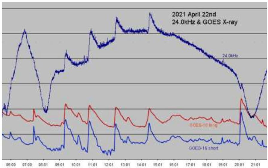
Mark has added the GOES X-ray data to his recording that also includes the later C8.5 flare caught on the 24 kHz signal. Colin Clements noted several radio bursts at 151 MHz, shown below. They are all following the C2.5 flare, although a connection is not clear. They were not detected at 408 MHz.
