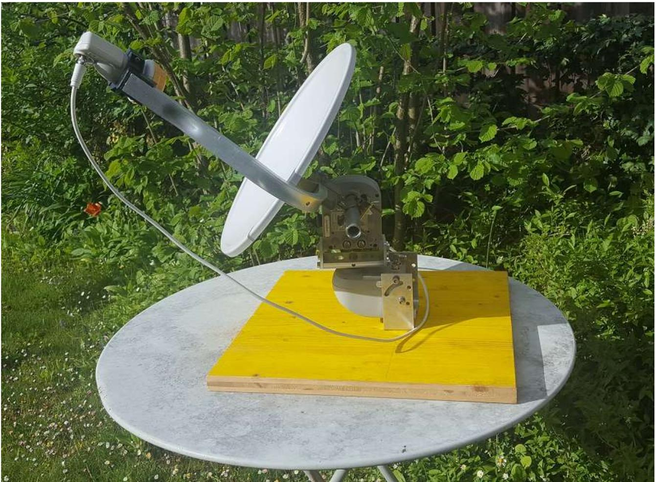
Fig. 1: Small 37 cm diameter offset dish antenna with a Ku-band LNB attached to two orthogonally mounted satellite dish rotors.
