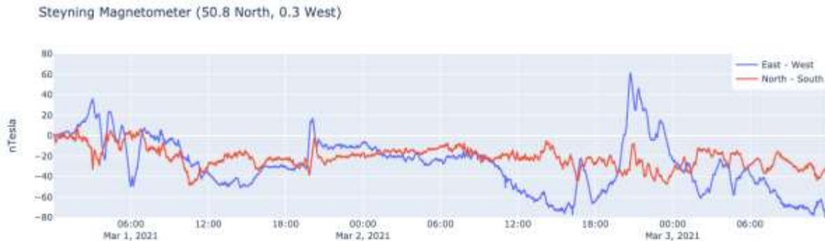
A period of strong disturbance can be seen in the evening of the 2<sup>nd</sup> with a large variation in the east-west component. Nick is located near the south coast, and so a comparison with the Mull magnetometer of Roger Blackwell, nearly 6 degrees further north, is of interest:
