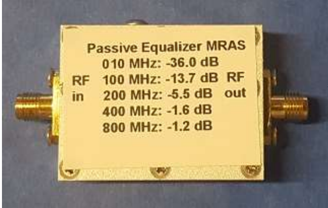
Fig. 5: Final product with cover mounted, a passive equalizer. Attenuation is on the order of -20 dB per decade.
