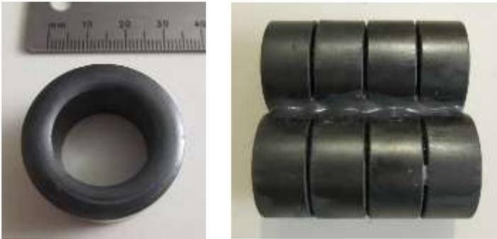
Figure 2 ~ Left: Fair-Rite toroid core, p/n 2675821502; Right: Binocular core formed from eight toroids in two rows. The cores in each row are first glued with superglue and after curing the two assemblies are then glued together with epoxy. ©2020 W. Reeve
