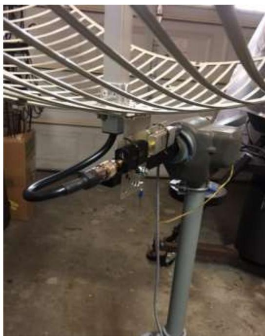
Figure 4 – Coax twisted once to meet LNA- SDR tandem, attached with zip ties near to rotation axis so USB cable gets minimal torsion when motor rotates.
