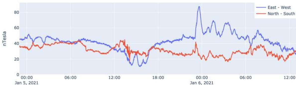
This recording by Nick Quinn shows the CME arrival just before midnight on the 5<sup>th</sup>, following a day of mild disturbance from the CHSS. Nick is using a fluxgate sensor buried 0.6m underground to reduce thermal effects. The disturbance faded out during the 6<sup>th</sup>. The second CME / CHSS combination arrived on the 11<sup>th</sup>, shown here by Roger Blackwell:
