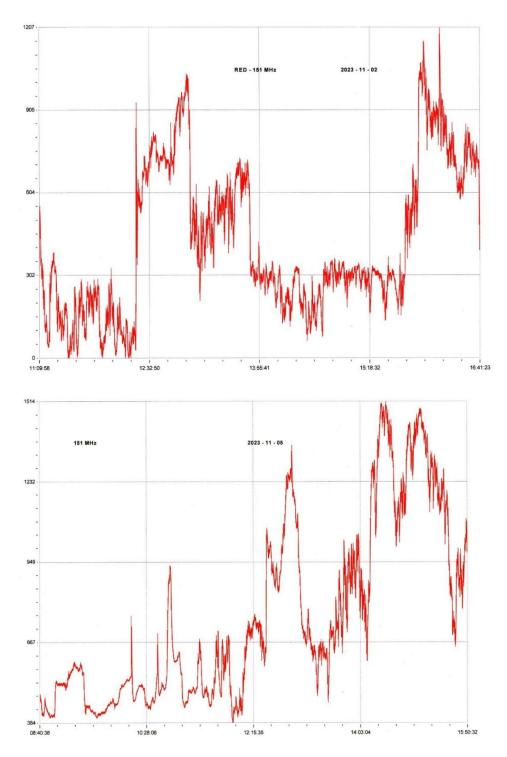
Colin Clements recorded some significant 151MHz solar noise during the strong flares on the 2<sup>nd</sup> and 5<sup>th</sup>. The aerial is now loft mounted and horizontally polarised, which seems to give a wider beam width for a fixed azimuth aerial. It is tricky to identify individual flares, as there were also plenty of smaller events that we did not record.
