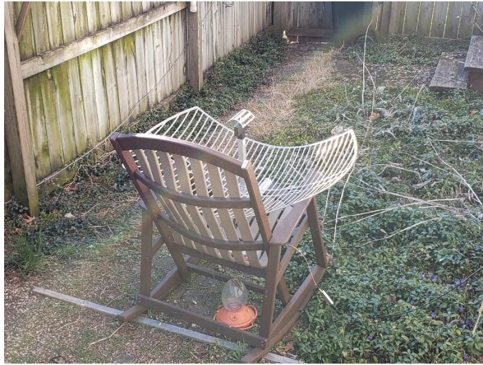
WiFi Antenna Used for H1
