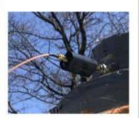
Nooelec Smartee SDR mounted on Large Heat Sink for Temperature Stability
