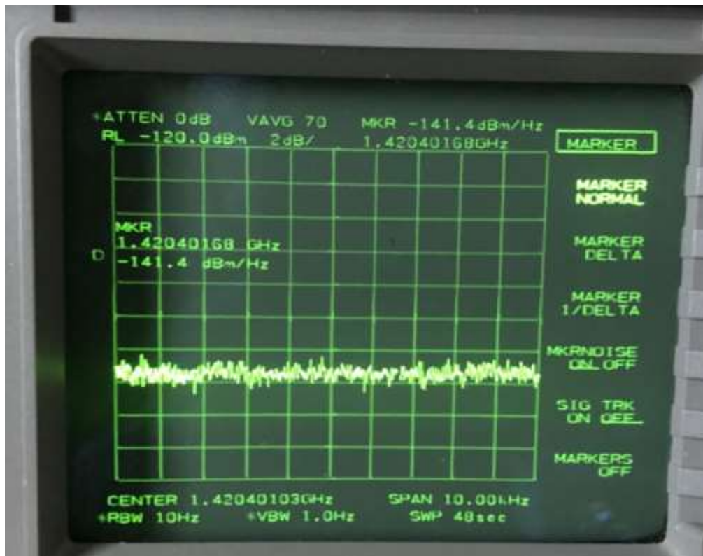
Figure 6. Spectrum analyzer Noise Measurement (100 Sweeps)
