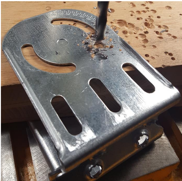
Figures 4a, b ~ Circular slits for antenna mounting need to be extended by about 10 mm, such that the offset angle of the antenna can be fully compensated for. Drill a whole and file it wide enough as depicted in figure 4b (red arrows).
