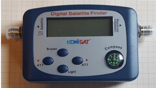
Figure 4 ~ Digital Satellite Finder HDMiSAT SF-9509C contains a digital display, an internal amplifier and an attenuator. The compass at bottom-right can be used to roughly set the azimuth of the telescope antenna.
