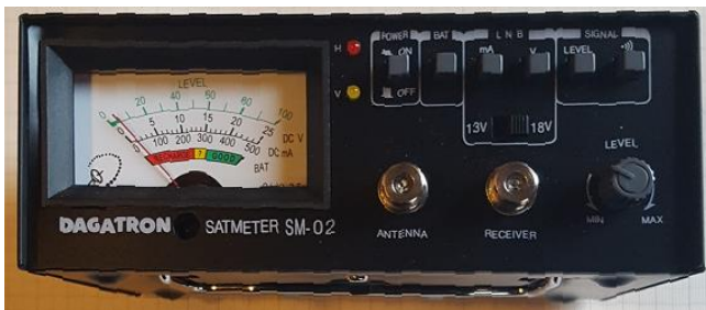
Figure 3 ~ Dagatron SATMETER SM-02 has an analogue display and works fine down to about 10.6 GHz. The unit is expensive because it contains a battery and allows control of the LNB polarization and measurement of the LNB voltage and current.
