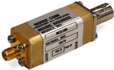
Figure 1: Calibrated semiconductor noise source to perform Y-factor and noise figure measurements. This type provides +33 dB ENR while another one used for CALLISTO measurements provides +15 dB ENR. The voltage source is +28 Vdc.
