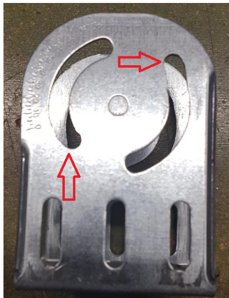
Figures 4a, b ~ Circular slits for antenna mounting need to be extended by about 10 mm, such that the offset angle of the antenna can be fully compensated for. Drill a whole and file it wide enough as depicted in figure 4b (red arrows).
