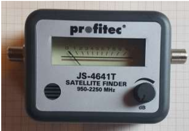
Figure 2 ~ Satellite Finder JS-4641T from Profitec with an analogue display meter and beeper. This unit works fine for frequencies above about 11.15 GHz but it is not usable at lower frequencies due to high attenuation and spurious signals. The knob at lower-right marked dB is used to adjust the sensitivity of the display and beeper.
