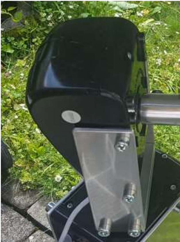
Figure 3 ~ Detailed view of elevation rotor on top of the azimuth rotor.
