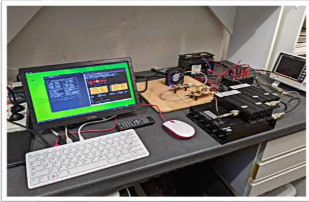
Figure 6: RPI400-Based Vela Pulsar Observation System
