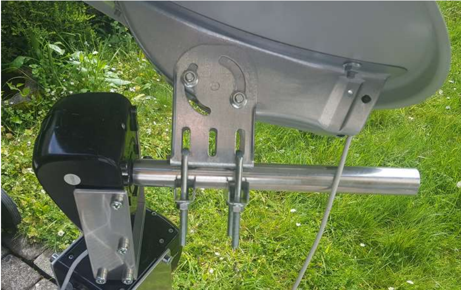
Figure 5 ~ Install antenna clamping adapter as close as possible to the elevation rotor to minimize moment on the elevation axis. While the axis is pointing west, mount dish such that feed arm and coaxial cable are also on the west side. Tighten the 4 hex-nuts with a wrench.
