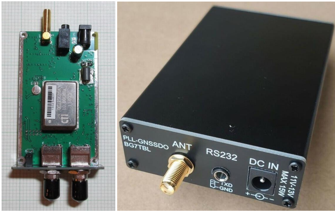
Figure 7.a ~ Left : System PCB, top view showing the OXCO (rectangular silver can in the middle), which is the same model as used in the SatTime GDO. Most components are underneath and not visible in this view. The output BNC-F connectors for the 10 MHz sinewave and 1 PPS and the status LEDs are at the bottom of the image. The antenna input, 3.5 mm serial port jack and dc power input jack are at the top of the image. Right : View of the antenna input, 3.5 mm serial port jack and 12 Vdc input jack panel. The transmit and receive pins on the RS232 (EIA-232) connector are reversed from convention. PCB dimensional tolerances are not particularly good – the nuts on the RF connectors cannot be tightened without warping the panels; the PCB should be redesigned or shims should be used.
