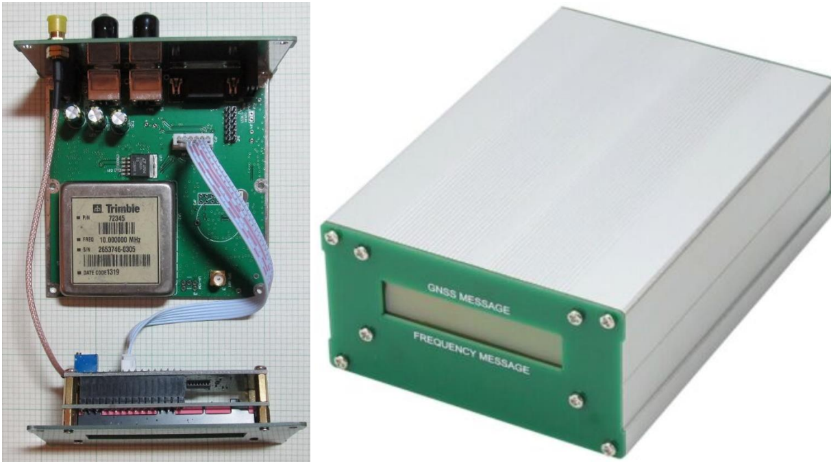
Figure 3.a ~ Left : System PCB connected by a ribbon cable to the LCD at bottom of image. Most components are underneath the system PCB. The Trimble OCXO is the large square can in the lower-left of the PCB. Note the well-used and worn appearance of the oscillator. The outputs, antenna input, dc power input jack, serial port interface and LED indicators are on the back panel at the top of the image. The outputs are 1 PPS and 10 MHz sinewave. Right : View of the front panel with the LCD (unpowered).
