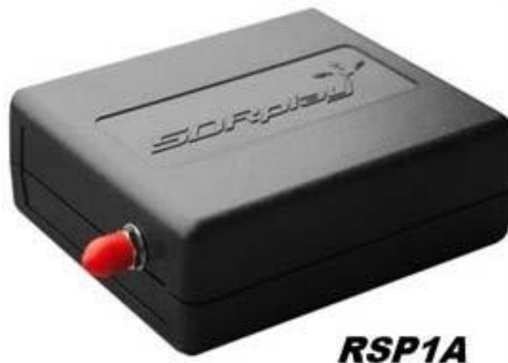
Figure 4. The JOVE team has had considerable success with the SDRPlay RSP1A unit and will provide support for using this instrument for our radio astronomy program. Not all SDR types can be supported, but it is our intent to provide support for some other SDRs as they become available during this period of rapid SDR development.
