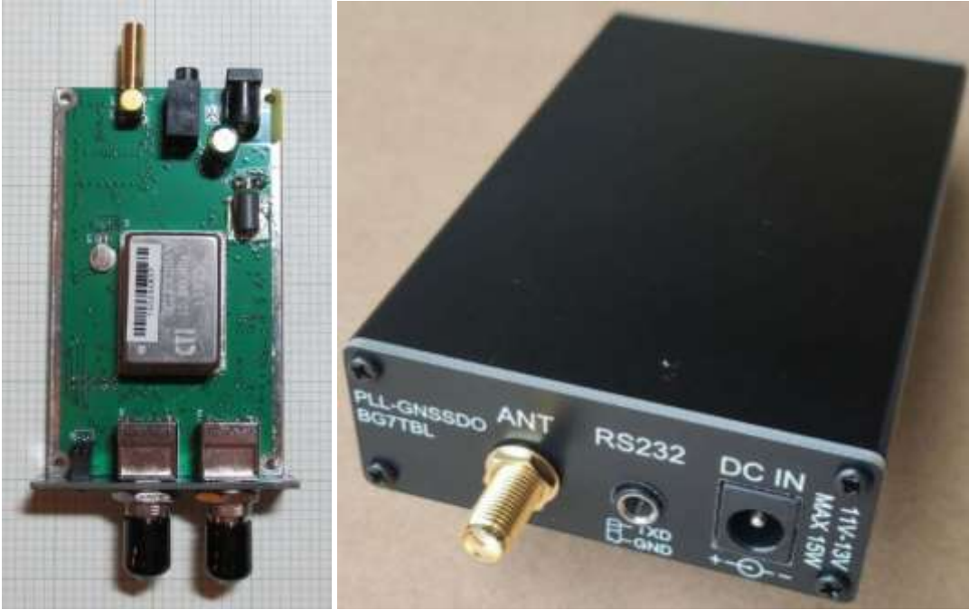
Figure 7.a ~ Left : System PCB, top view showing the OCXO (rectangular silver can in the middle), which is the same model as used in the SatTime GDO. Most components are underneath and not visible in this view. The output BNC-F connectors for the 10 MHz sinewave and 1 PPS and the status LEDs are at the bottom of the image. The antenna input, 3.5 mm serial port jack and dc power input jack are at the top of the image. Right : View of the antenna input, 3.5 mm serial port jack and 12 Vdc input jack panel. The transmit and receive pins on the RS232 (EIA-232) connector are reversed from convention. PCB dimensional tolerances are not particularly good – the nuts on the RF connectors cannot be tightened without warping the panels; the PCB should be redesigned or shims should be used.
