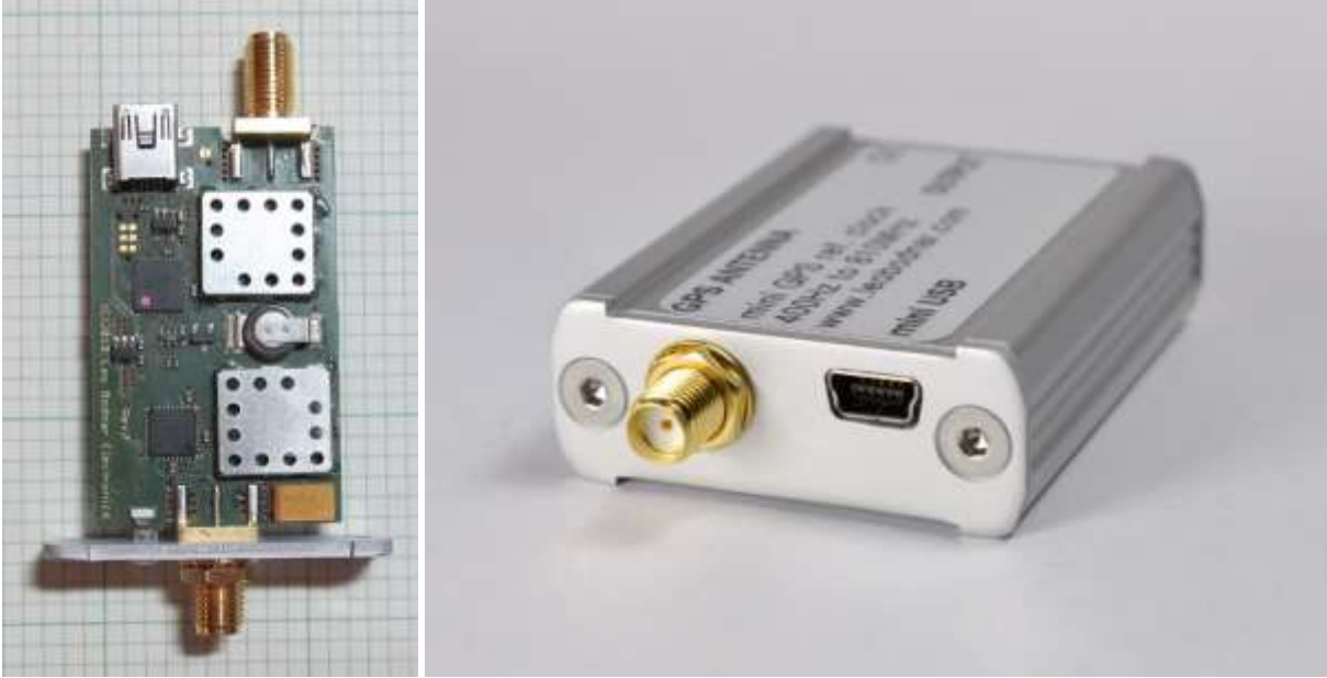
Figure 6.a ~ Left : System PCB. The TCXO is presumably under one of the metal shields. The output is at the bottom and the antenna input and Mini-USB connector are at the top of the image. The only output is a variable frequency squarewave the frequency of which is set by the user; I set my unit to 10 MHz; Right : View of the antenna input and Mini-USB connector panel. Image source: leobodnar.com
