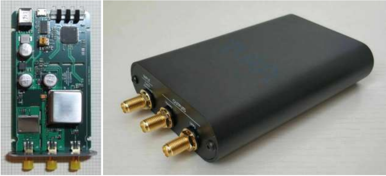
Figure 5.a ~ Left : System PCB for one of the two units evaluated. The OCXO is the large, square silver can; note the newer appearance than the BG7TBL-D and SatTime (before replacement). The 10 MHz and 1 PPS outputs and antenna input are at the bottom, and the dc power jack, Micro-USB connector and LED indicators are at the top of the image. Right : View of the output and antenna input panel. The outputs are 10 MHz sinewave and 1 PPS.
