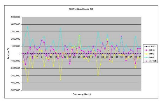
Illustration 8: This is the result of a Quad Cross Correlation starting at 0 Hertz to 100 Hertz (in 2 second bins). When Angle, Real, Imaginary, and Magnitude values (Jansky measures) are positive there may be a significant correlation between the two frequencies and a possible indication of a mixture of polarizations at different amplitudes, and altitudes on the sun.
