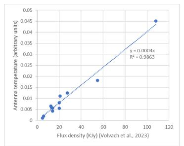
Figure 3: correlation between measurements of the 1 metre dish and reported flux density of the flare.
