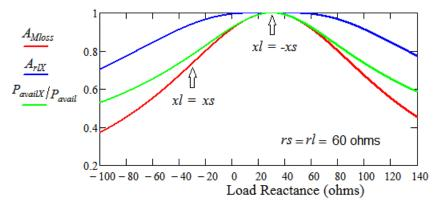
Figure 3. Loss v Load Reactance; Total loss (red), Available Power (green), Resistive Mismatch Loss (blue)
