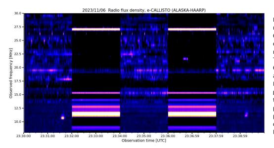
Figure 1 ~ The 2minute On/2-minute Off cycle of the IRI is clearly seen in this 10 minute spectrogram. The responses of the Callisto spectrometer and antenna Front End Electronics were grossly nonlinear due to their close proximity to the powerful IRI. Image courtesy of Christian Monstein
