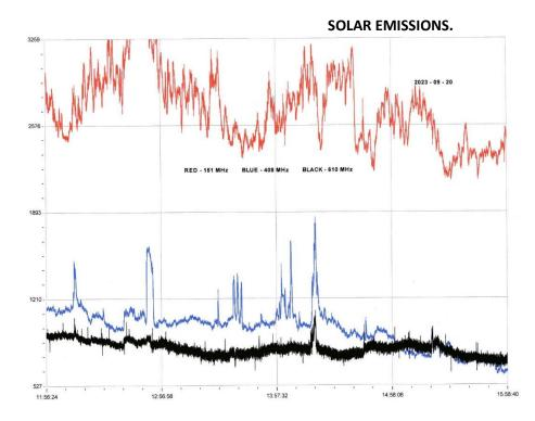
Colin Cements' recording from the 20<sup>th</sup> shows some significant noise, particularly at 151MHz (red) through the afternoon. The M8.2 flare at 14:20UT matches with the strong 408MHz (blue) spike, along with a much weaker spike at 610MHz (black).
