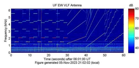
Figure 4 ~ HAARP induced ULF and VLF emissions received at
