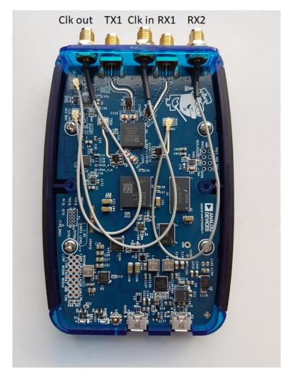
Figure 1: Modified ADALM Pluto (Rev. C board)
