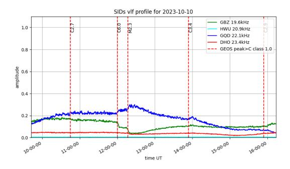
The recording by Mark Prescott from the 10<sup>th</sup> shows the stronger of the two M-class flares recorded. The M2.3 flare has interrupted the earlier C6.0 flare, giving good mirror image SIDs at 19.6kHz and 22.1kHz. 23.4kHz has remained largely unaffected, with just a very minor drop in signal level. Different active regions produced these flares, although they were less than 10 degrees apart. The later C3.4 flare is also well shown at 22.1kHz.
