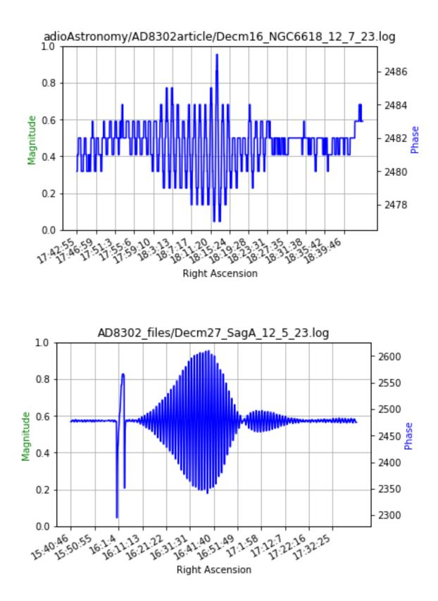
This last one is a combination of the Sun and Sagittarius A. The Sun was coming into Sagittarius and was at -23 Declination. Sag A is at -27 declination. The beam width of the dishes is ~5 deg. Also, the Sun is so strong that it shows up in things 30 deg away.
