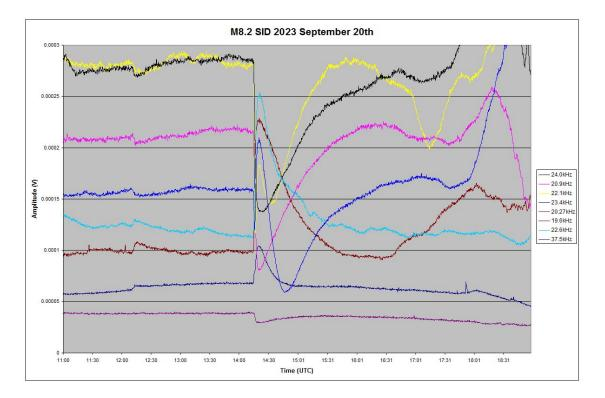
The M8.2 flare peaking at 14:22UT on the 20<sup>th</sup> was one of the strongest and shows a good variety of SID shapes on this recording by Mark Edwards. The chart runs from 11:00 to 19:00, and just shows the much weaker C3.4 flare at 12:13, the C4.2 at 18:04 and C5.5 at 18:40. The last two show best on the Atlantic path at 24kHz, dark blue on the chart.
