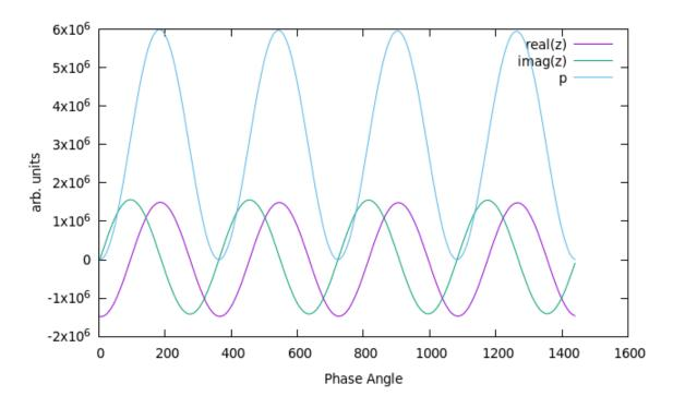
Figure 3: Recorded phase and power signal
