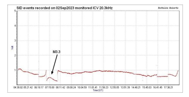
The flare started just before the sudden drop in signal level, but the peak sits neatly near the middle before the signal rises again and the flare fades out. Excellent timing! Isola di Tavolara is a small island near Sardinia, due south of Milan, at 9 degrees east.
