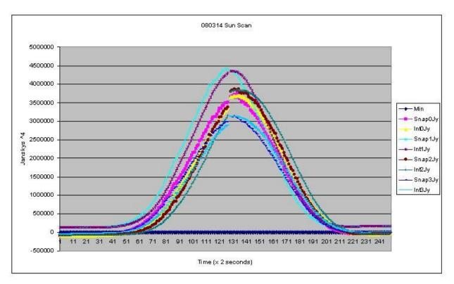
Illustration 6: Channels 0 - 3 during a Sun Scan. There is pause near the peak where a 2 minute snapshot of data was taken for the Quad Cross Correlation routines to examine the polarization of Vertical, Horizontal, Right Circular and Left Circular polarization measured in Janskys.
