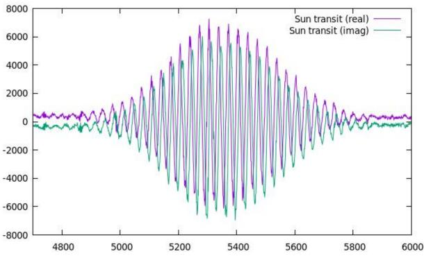
The result (i.e. the fringes) can be seen in fig.5. The fringe time is ~ 37 seconds.
