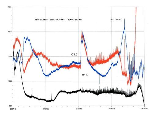
Colin Clements' recording from the 2<sup>nd</sup> shows the M1.9 flare at 23.4kHz (red) and 21.75kHz (blue) with very strong SIDs, along with the much weaker C3.0 flare. The 21.75kHz response appears to be a spike and wave
