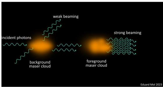
Figure 5: illustration of maser beaming due to maser clouds overlapping along the line of sight. Note that the foreground cloud can only amplify the radiation from the background cloud if both clouds are moving at the same velocity along the line of sight. If the foreground cloud is moving at a different velocity with respect to the background cloud, the radiation from the background cloud is slightly red- or blueshifted away from the water line frequency and thus cannot be amplified.
