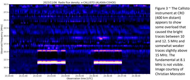
instrument at CRO (400 km distant) appears to show some overload that caused the bright traces between 10 and 12. 5 MHz and somewhat weaker traces slightly above fundamental at 8.1 MHz is not visible. Image courtesy of **Christian Monstein**
