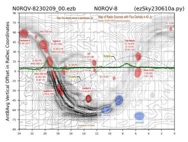
The green line represents detected hydrogen of a drift scan across the sky at a certain elevation in RaDec.
