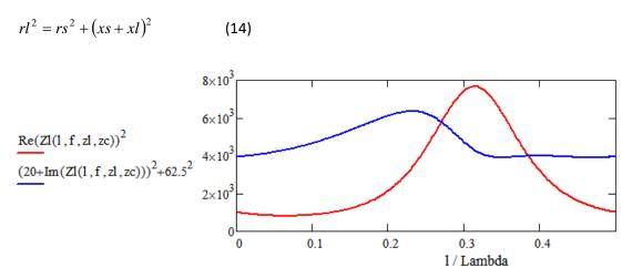
Figure 7. Confirmation of Optimum Transmission Line Lengths.
