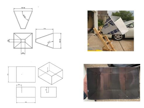
Figure 1: Dimensions and Photos of Antenna
