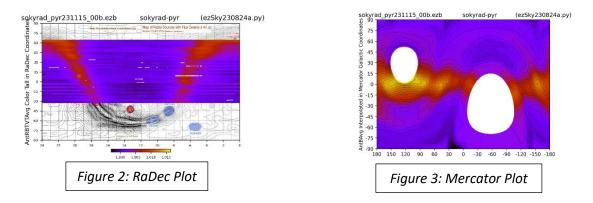
The white areas in the Mercator are points in the sky not visible from my location. Figure 2 clearly shows the galactic hydrogen, and it is plotted against known radio sky maps for comparison. The data shows some striations in some elevations, due to a change in the waveguide construction part way through the survey.
