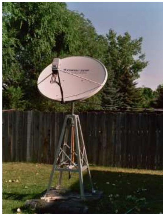
Illustration 1: A 90 centimeter offset dish with Invacom QPH-031 dual polarity dual frequency LNB.
