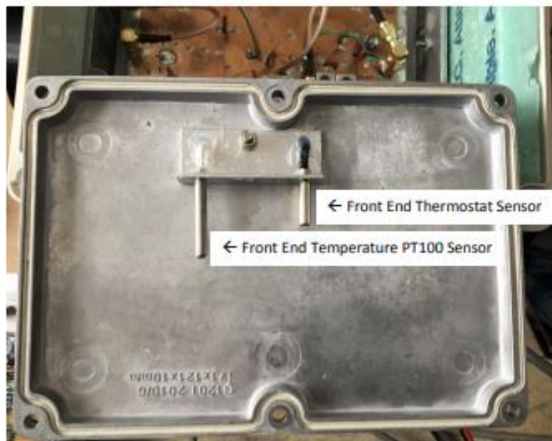
Figure 6. Neutral Hydrogen Receiver Front End Temperature Probes (inside cover)
