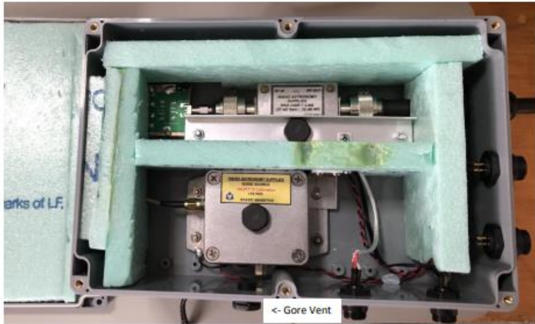
Figure 3. Neutral Hydrogen Receiver LNA Thermal Insulation
