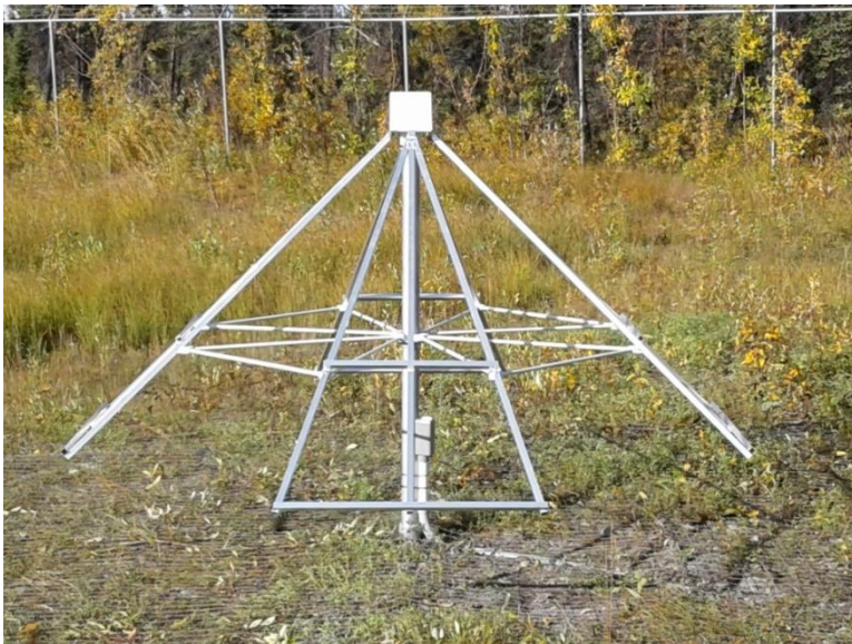
Figure 2 ~ LWA Antenna at HAARP Radio Observatory soon after installation in September 2021. The antenna is an active, tied-fork, crossed-dipole, 1.5 m high with the Front End Electronics (FEE) in the square hub enclosure at the top. The antenna and associated spectrometers are collocated on the science pad with the Modular UHF Incoherent Radar (MUIR) at the HAARP facility. The chain-link fence that surrounds the science pad can be seen in the background about 25 m away. Image © 2021 W. Reeve.
