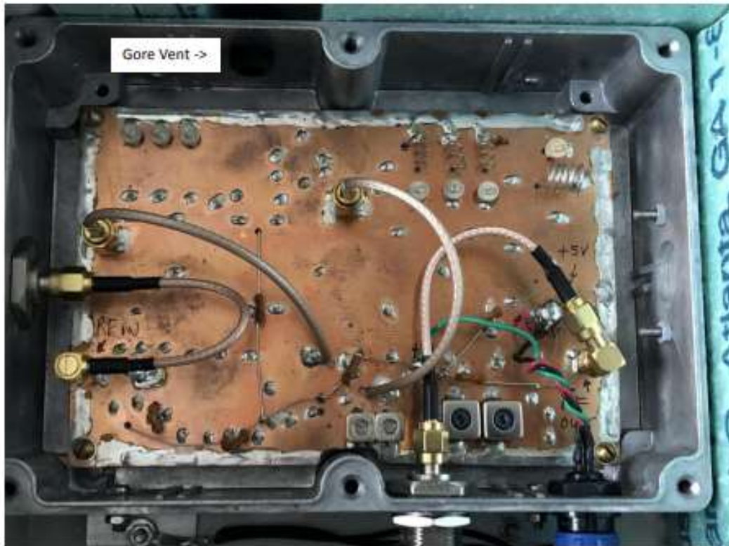
Figure 5. Neutral Hydrogen Receiver Front End Internal View (cover removed)
