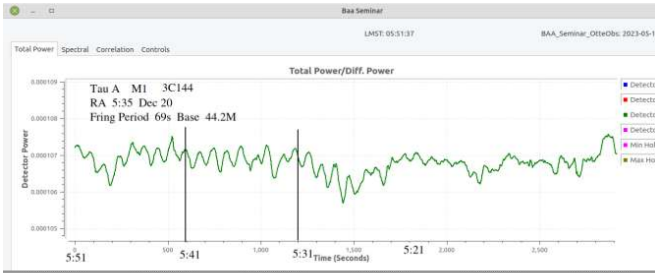
Image 4: This is a little different graph presentation using a screen shot of BAA Seminar total power screen itself. Taurus A is not giving the “perfect” profile shot but all the features shown in the Cyg A graph are here also. The fringes are harder to count but I get between 8 and 9 so 600/8.5 = 70.5 s. The phase change imperfection is at about 1000 on the seconds scale or maybe the tall one at 500. Can’t get much brightness data off of this.
