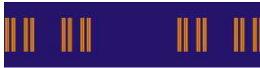
Figure 5. A Cantor Linear Fractal Array
