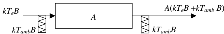
Figure A1. Noise Temperature of an Attenuator; Injected Noise power Doubles Output Power
