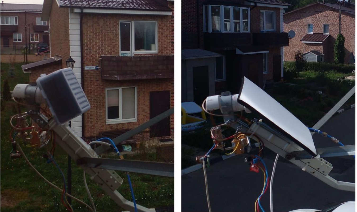
Figure 3: Flux calibration of the 80 GHz IBT: a plastic box (a calibration load) with a foam RF absorber sheet inside (left) and just a RF-absorbing sheet covering the feed (right).
