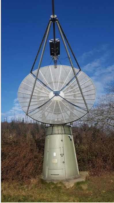
Figure 10 ~ 5m parabolic dish at radio astronomy facility of ETH Zurich in Bleien. Box behind feed contains band pass filters and a low noise amplifier. While tracking the Sun, the entire antenna rotates in azimuth and in elevation controlled by a standard Windows computer. The estimated gain of is 45 dBi in L-band. Tower carrying the dish is a spotlight structure from WW-II. The shade of the focal plane unit in the dish center proves that the dish is tracking the sun. This dish antenna was used to produce the light-curve plot, shown in figure 15. Image courtesy of C. Monstein.
