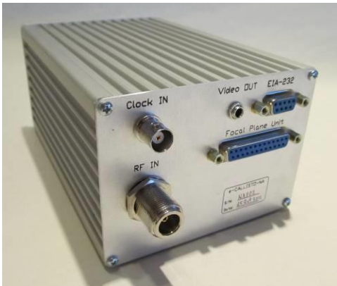
Figure 6 ~ Callisto is a channelized sweep-frequency receiver. In most configurations, the channels are swept at a rate of 800 channels/s, but this can be extended to 1000 channels/s when the Callisto is connected to a 1 MHz reference clock source. The Callisto instrument dimensions are 200 x 110 x 82 mm and it weighs 0.9 kg. It is powered by a 12 Vdc power supply and controlled through an EIA-232 interface. Image ©2012 W. Reeve
