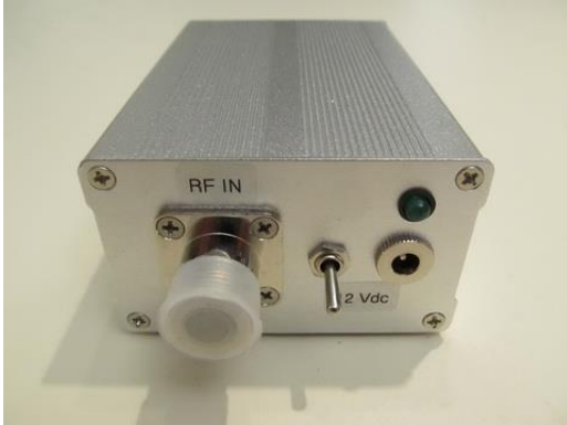
Figure 8 ~ Inexpensive amplifier package made with a modular low noise amplifier. Dimensions are 110 x 77 x 47 mm and average measured noise figure across the frequency range 45 to 870 MHz is 0.8 dB. This unit requires 12 Vdc at 40 mA, and it can be powered through the coaxial cable using a pair of bias-tees or directly with a separate power cable. It is not weatherproof so it must be covered if there is rain during the eclipse. Image ©2015 W. Reeve
