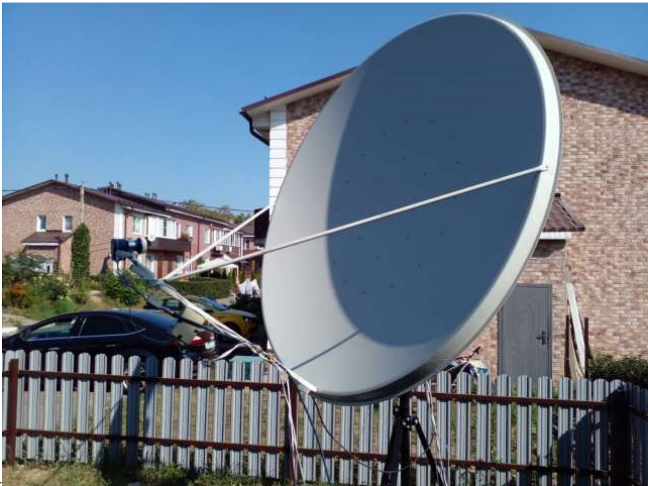
Fig. 1. Outdoor observation setup, dish D=1.8 m, automatic Az-El tracking. Location near Moscow (N56.146254, E37.496530).
