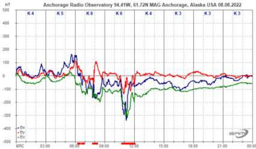
Figure 13 ~ On 8 August, geomagnetic disturbances from coronal hole high-speed streams led to storm conditions with K-index K5 or higher in the 0300-0600, 0600-0900 and 0900-1200 synoptic periods. Earth’s magnetic field showed erratic deviations during these periods but quieted down after 1200.
