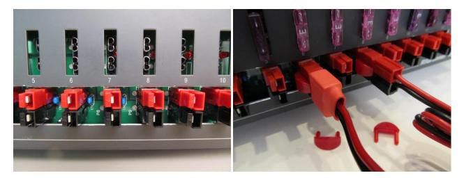
Figure 4. <u>Left</u>: Cover in place and modifications completed. Now, the retention clips can be inserted on either side to hold the connectors in place. <u>Right</u>: Retention clips in-place on two of the connectors with a couple extra clips immediately below. Only a little dexterity is needed to fit the clips, which securely hold the connectors in-place.
