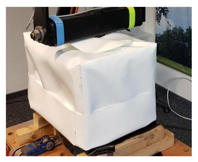
Fig 6: Water protection cover for azimuth drive
