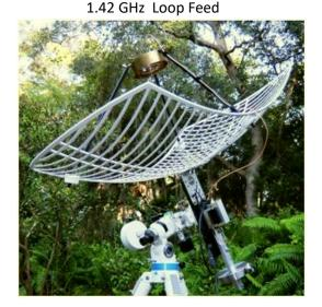
As an experiment, side panels were added to improve the SNR of the antenna, The intent was not to increase the size of the dish and gain signal enhancement, but to shield the loop-feed's 'over-illumination' pattern from ground noise.
