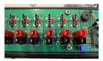
Figure 2. Removal of LED current limiting resistors (throughhole types). The resistor leads have been cut and the bodies discarded. Compare to left side of figure 1.
