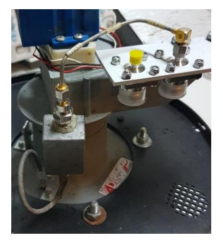
Fig 1: Feed horn with LNA and adapters
