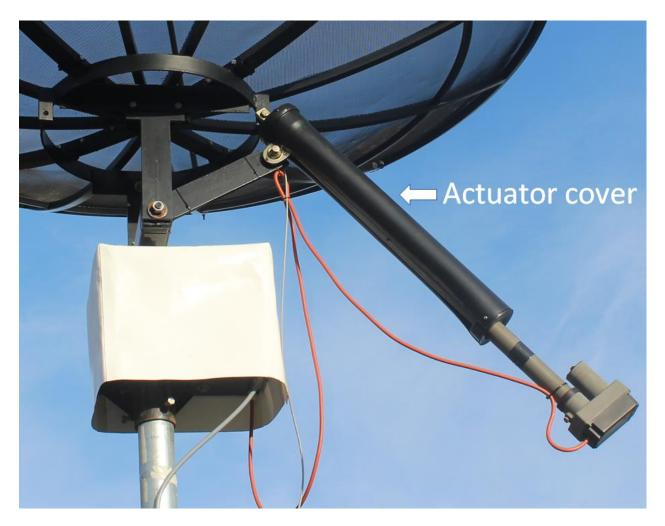
Fig. 8: Linear actuator with cover
