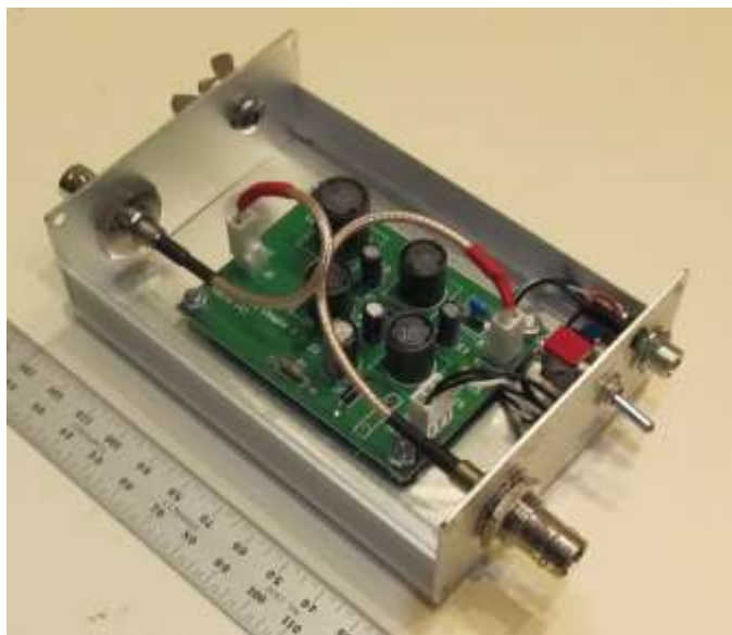
Figure 1 ~ Power coupler for VLF and LF applications with multi-stage lowpass filter and power controls in an extruded aluminum enclosure. This is one of several variations built over a 3-year period for the HP 10509A loop antenna. It uses RG-316 coaxial cables from the BNC-F bulkhead connectors to the PCB, but twisted pairs work just as well at the low frequencies of operation and have been used in other variations. Image © 2021 W. Reeve
