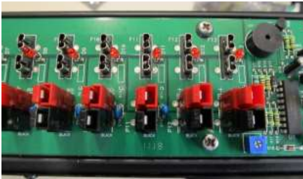
Figure 2. Removal of LED current limiting resistors (through-hole types). The resistor leads have been cut and the bodies discarded. Compare to left side of figure 1.
