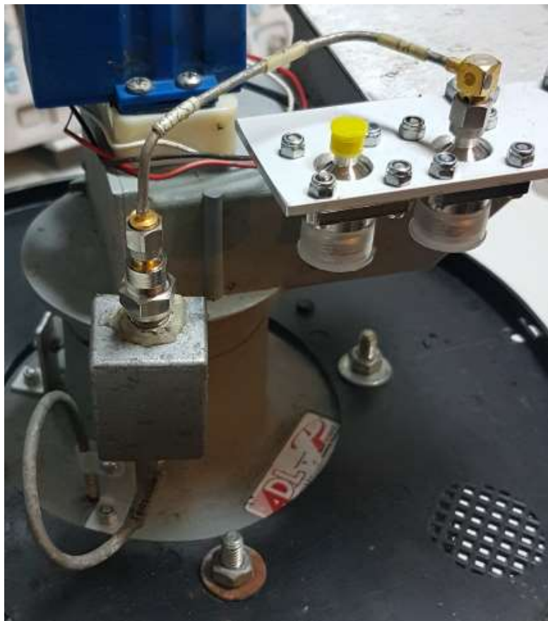
Fig 1: Feed horn with LNA and adapters
