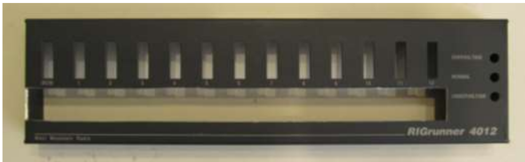
Figure 3. Cover for a 12-circuit distribution panel. The metal webs between the PowerPole connectors have been removed with a nibbler tool. The fuse slots are immediately above the cutout area. Compare to the right side of figure 1.
