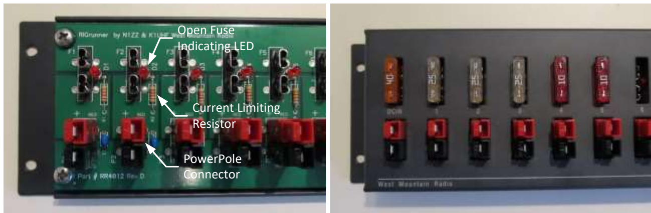
Figure 1. Left : Cover removed from a RigRunner distribution panel. The blown-fuse indicator LEDs on the printed circuit board can be seen just to the right of and between the two fuse blade sockets. The 1200 ohm current limiting resistors are visible below and to the right of the LEDs. Right : The LEDs are invisible under normal lighting conditions. A faint glow can be seen when a fuse blows and the ambient light is low. These images show early versions of the distribution panel with through-hole resistors and LEDs. Later versions use surface mounted devices (SMD).
