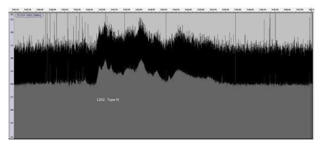
Colin Briden recorded a type III burst starting at 12:02UT on the 1<sup>st</sup>:
