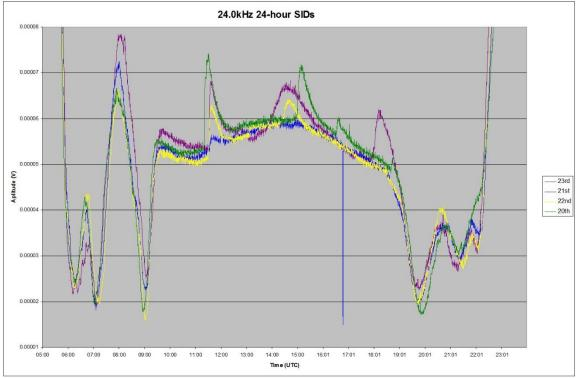
Mark Edwards noticed an apparent 24 hour repetition of flares on the 21<sup>st</sup>, 22<sup>nd</sup> and 23<sup>rd</sup>. His recording shows the three days superimposed, all showing a SID within a few minutes of 11:36, and the 20<sup>th</sup> just 5 minutes earlier. Just pure chance I suspect!
