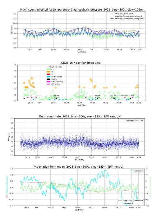
The data has been adjusted for temperature and atmospheric pressure as explained in the August edition. Muon counts can be seen to fall slightly following the stronger solar events as the solar wind speed and density increases.
