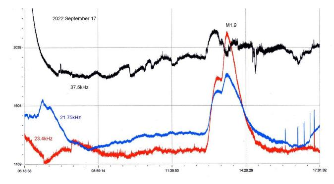
The 37.5kHz signal is tricky to interpret, but appears to show a peak matching the first peak at 21.75 and 23.4kHz, followed by a dip at the M1.9 peak. SIDs on other days do show a rise in signal strength from the 37.5kHz signal. The recording by Roberto Battaiola also shows a very similar SID response:
