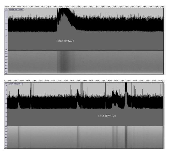
This 28MHz type III signal is from the 19<sup>th</sup>, peaking about 20dB above the background at 11:46 on the 19<sup>th</sup>. Its timing matches a C1.7 flare, although we did not record a SID from it.
