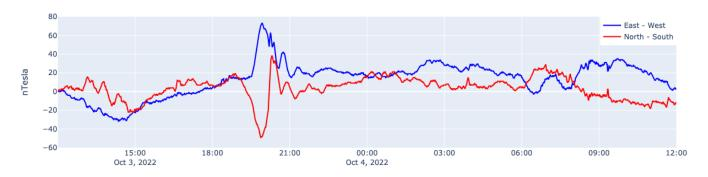
This recording from the 3<sup>rd</sup> and 4<sup>th</sup> by Nick Quinn shows a strong pulse around 20UT. It does not seem to be a CME impact, so is probably a shock in the solar wind. Recordings by Roger Blackwell show strong solar wind disturbances continuing on the 4<sup>th</sup>, 5<sup>th</sup> and 6<sup>th</sup>:
