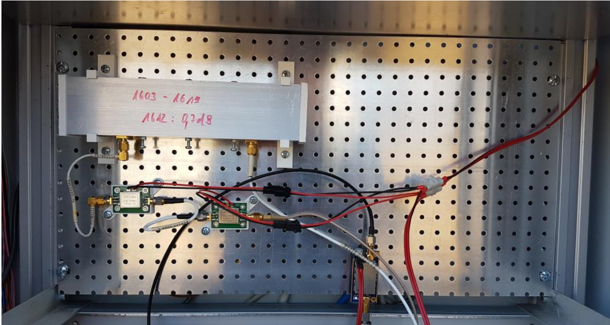
Fig 5: Different RF configuration for 1612 MHz
