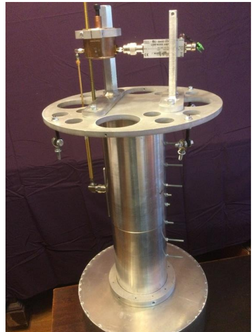
Figure 6b: Feedhorn with Choke Ring, Line Stretcher, Band Pass Filter, and Kuhne LNA
