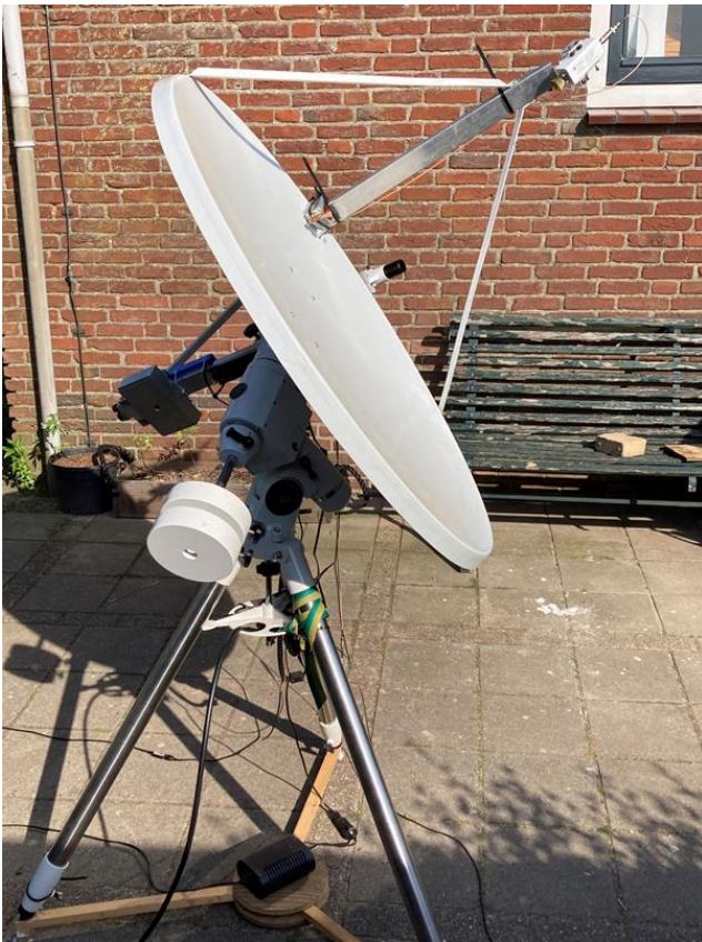
Figure 7: 1- metre offset dish on HEQ5 mount
