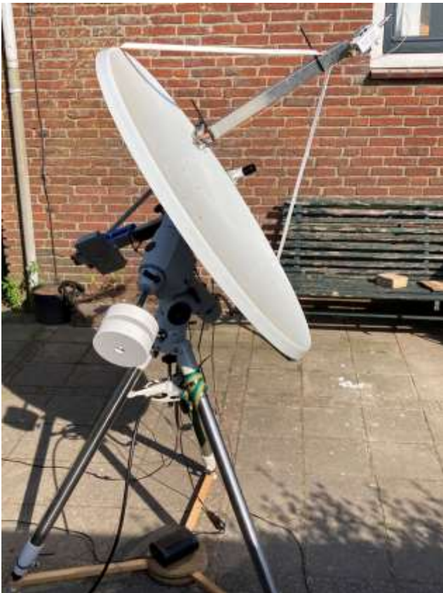
Figure 7: 1- metre offset dish on HEQ5 mount
