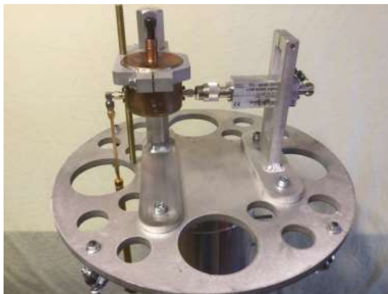
Figure 7: Highlighting the Filter (Copper Colored Device)
