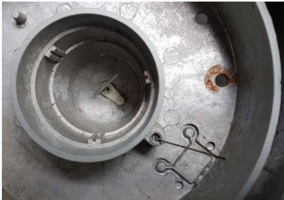
Figure 11: Detail view of the probes in the feed horn
