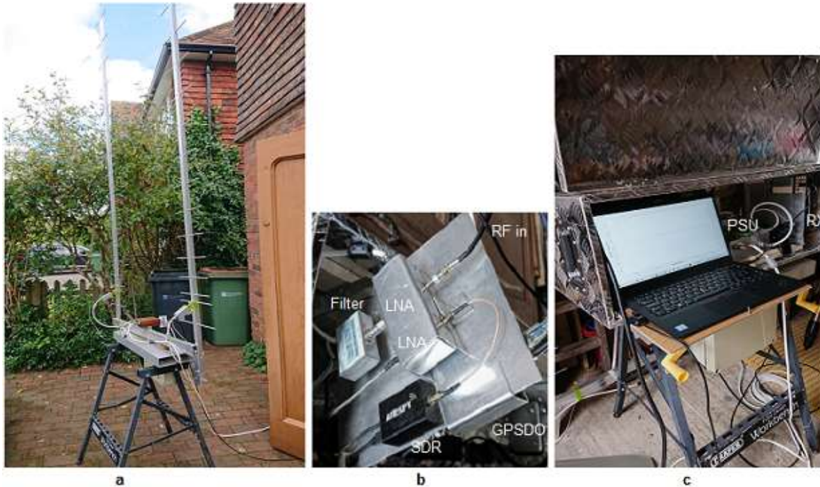
Figure 1. a) Antenna LNAs and Combiner. b) Receiver Panel. c) System Housing and Data Collection PC.
