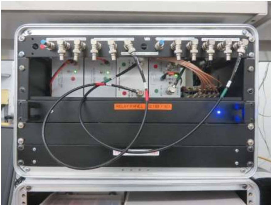
Figure 2 ~ All electronics were installed in an equipment cabinet (of the type used by musicians) and placed in the MUIR enclosure. The two Callistos are at the upper-left. Next to them, and in the middle, is the UPC-590L dual up-converter and to its right is the LWAPC-Q power coupler. The RF patch panel along the top of the cabinet is connected to two 6-port splitters on the far-right next to the LWAPC-Q. Immediately below is the LAN-controlled relay panel for remotely cycling the dc power to the Callistos. At the bottom of the cabinet are the 5, 12 and 15 Vdc power supplies. Not shown are the PC, LAN/WAN components and Uninterruptible Power System.
