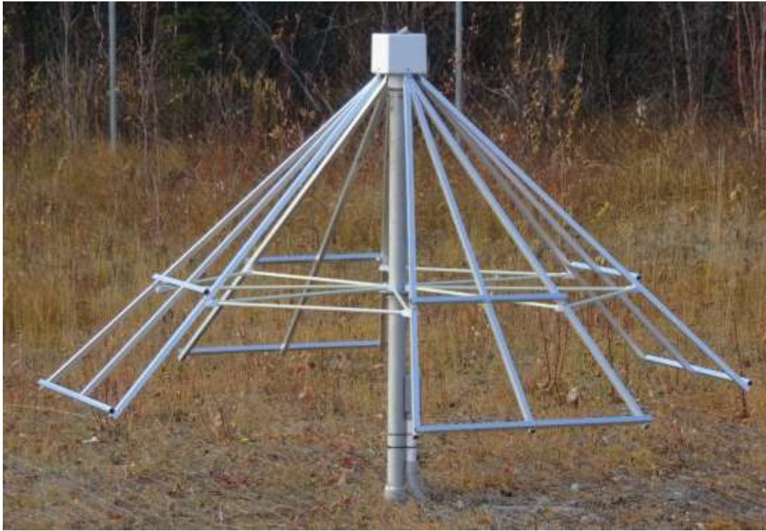
Figure 2 ~ LWA Antenna installed at the Modular UHF Incoherent Scatter Radar (MUIR) site on the HAARP facility. The antenna consists of aluminum, tied-fork, crossed-dipoles supported on a 1.5 m steel mast. Frequency range is approximately 10 to 100 MHz but is usable only to about 85 MHz because of FM broadcast station interference. Image © 2021 W. Reeve
