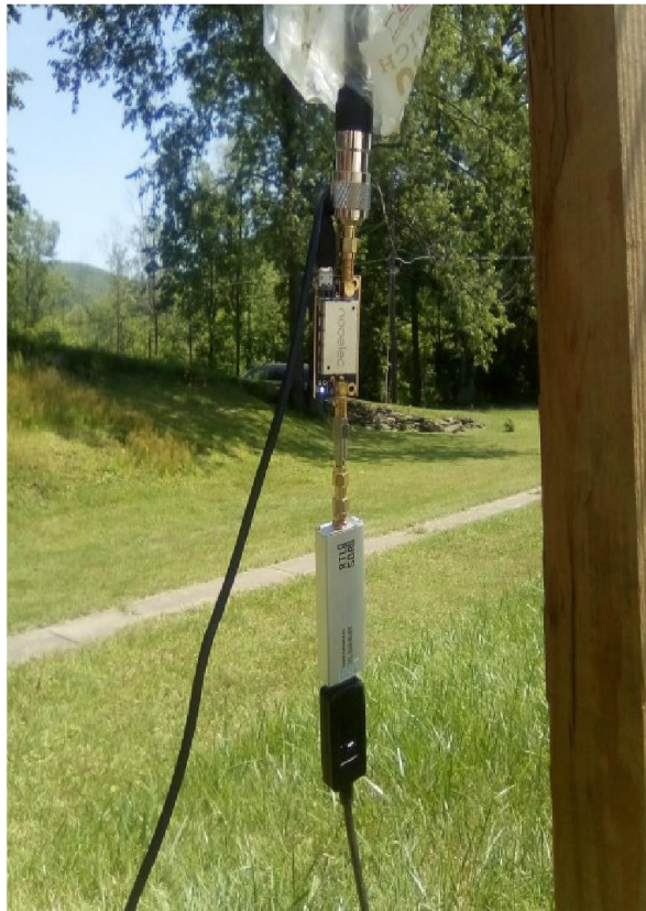
Figure 2: Close up view of the N - SMA adapter, LNA, DC Block, Dongle and USB Cables, note the plastic bag which is used to protect the electronics from rain.
