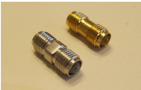
Figure 2 ~ nanoVNA SMA barrel connector (upper-right) alongside a high-quality connector. The brass nanoVNA connector has no flats for a wrench and cannot be properly torqued. The RF Industries model RSA-3404 nickel-plated brass connector shown next to it has flats for a 5.5 mm wrench. I made all connections involving the brass barrel connector finger-tight. Image © 2021 W. Reeve
