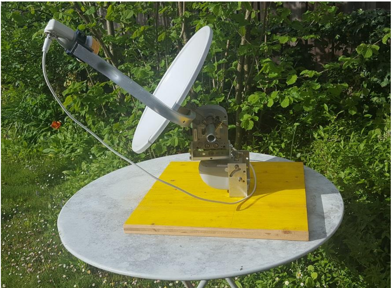
Fig. 1: Small 37 cm diameter offset dish antenna with a Ku-band LNB attached to two orthogonally mounted satellite dish rotators.
