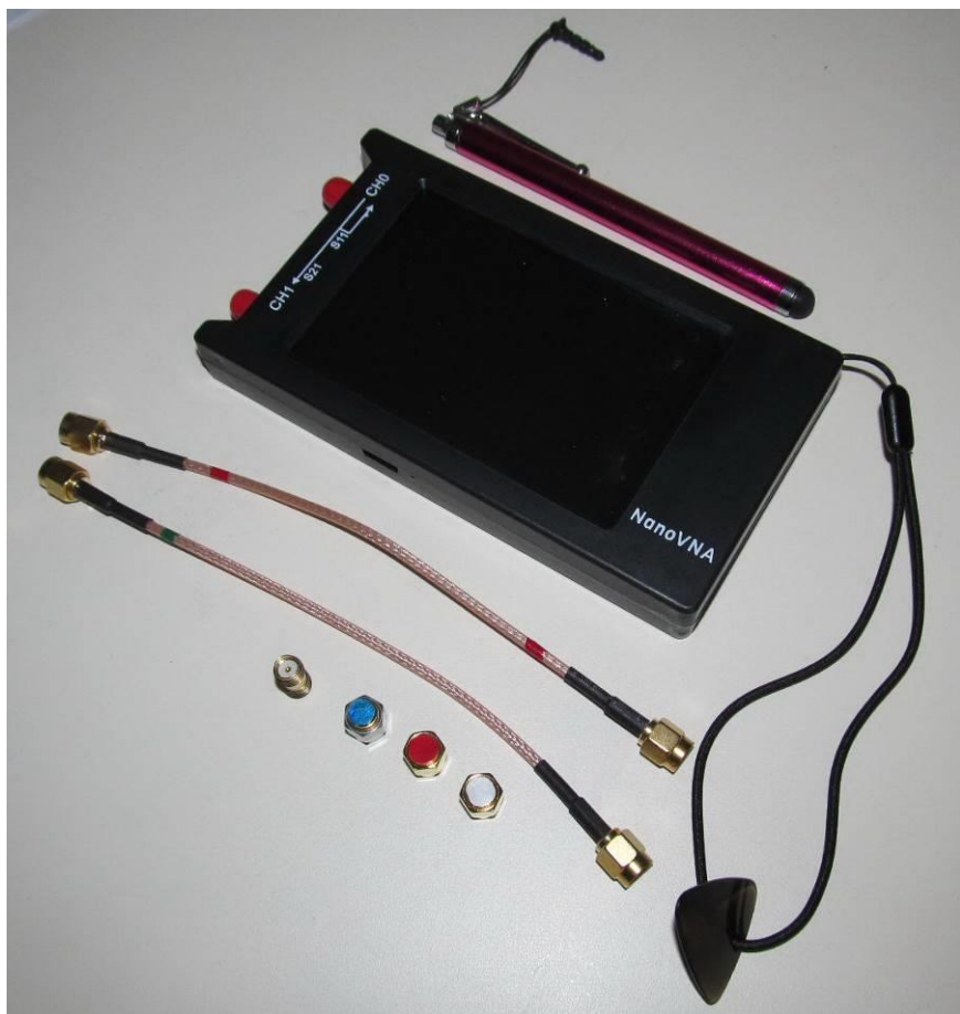
Figure 1 ~ nanoVNA-H4 and measurement accessories supplied with it. These include two RG-316, 150 mm long coaxial jumper cables with SMA male connectors, SMA male Open, Short and Load calibration standards, and an SMA female barrel connector. It also included a couple USB cables and a Quick Start Guide (not shown). Note the guitar pick on the lanyard to be used as a stylus. I prefer a soft-tip stylus and added the one shown above the unit. The calibration standards have an identical outward appearance, so I color-coded them with fingernail polish for easy identification: Blue = Load; Red = Short; and White = Open. The SMA barrel connector, seen to the left of the Load, is not strictly part of the calibration standards but is necessary for Thru calibration and when using the standards with cables or devices that have male connectors. I also marked the two coaxial jumper cables red and green for identification. Image © 2021 W. Reeve
