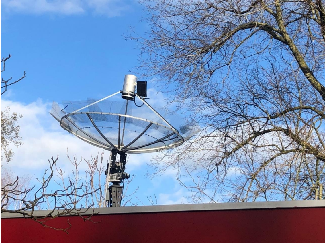
Figure 7: JRT, Job's Radio Telescope with extra mesh and rotator. Can feed and the LNA's/filters in black box
